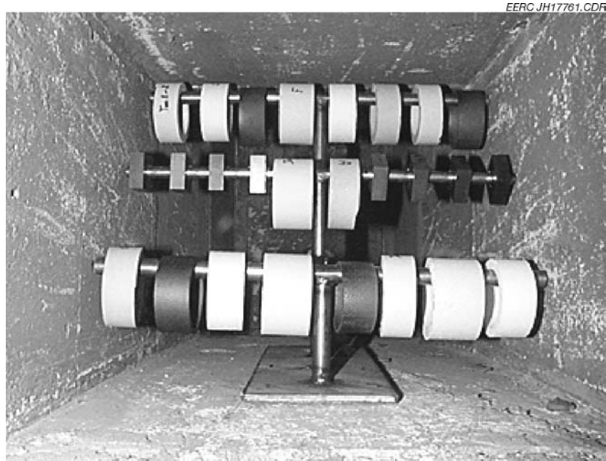
Figure 2. Material coupons in the convective pass of the SFS, viewed from the upstream side, before the March 2000 test.
