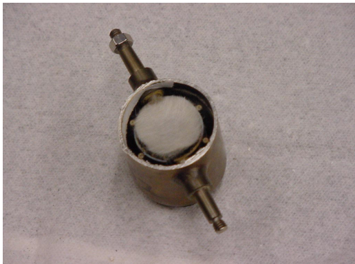
Reformer catalyst inlet flame arrestor / radiation shield
