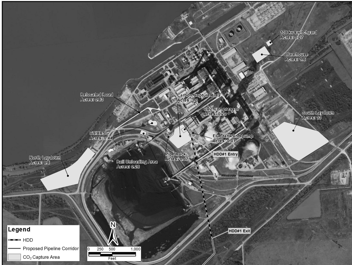
Figure 2-4. CO 2 Capture Facility Plot Plan
