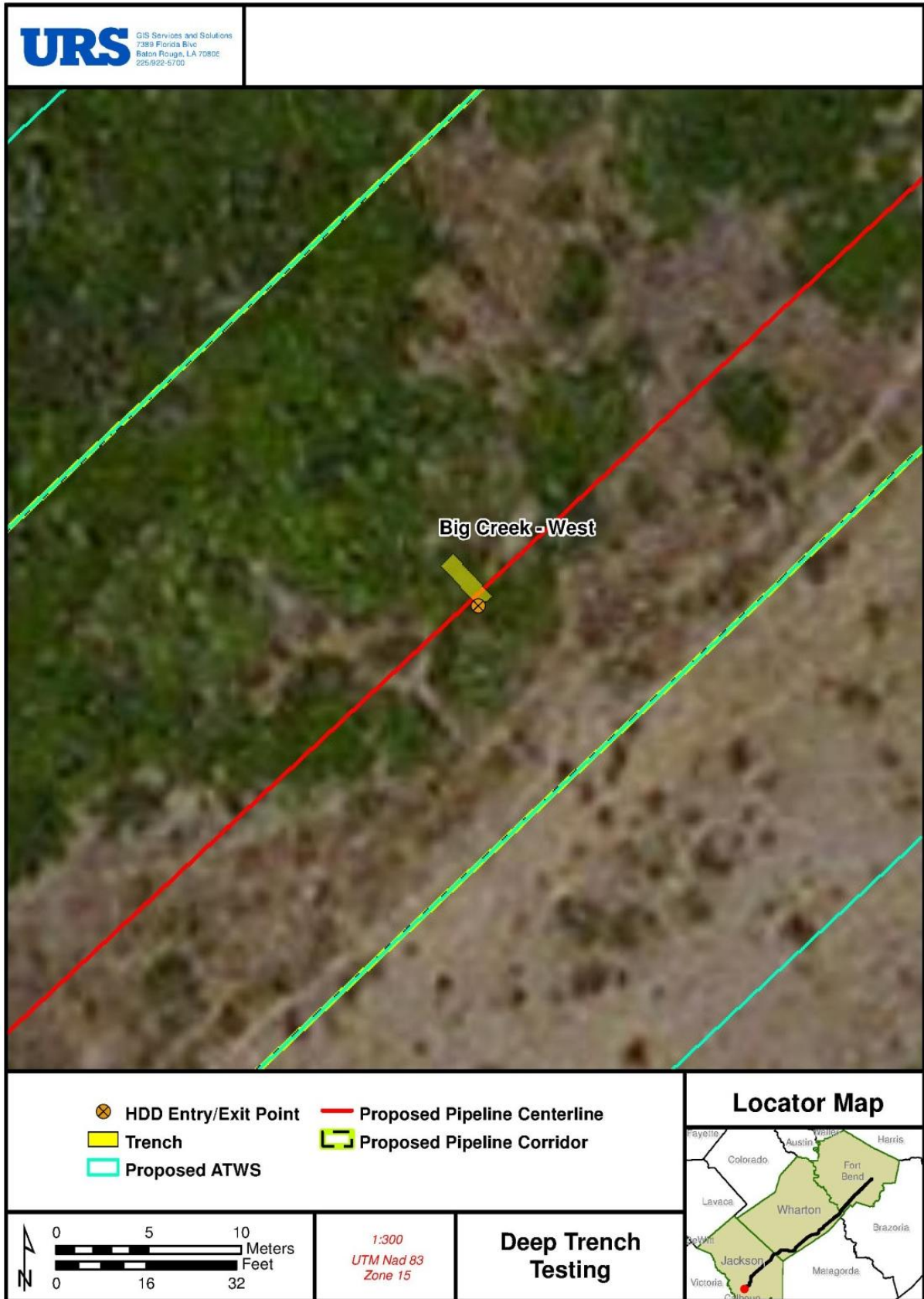
Figure 15: Big Creek - West HDD Planview
