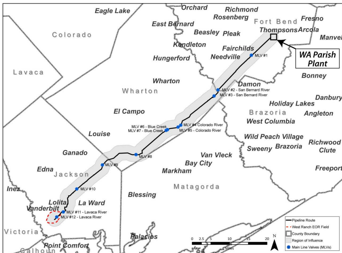
Figure F-1. Map of Planned Pipeline with MLVs between W.A. Parish Plant and West Ranch Oil Field
