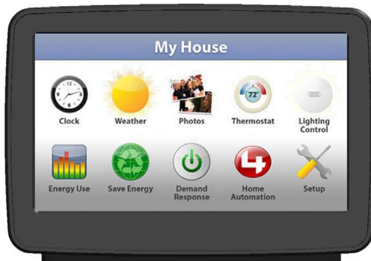
Figure 2. The consumer home energy display provides easy interface to several programs. Image of EMS-100 courtesy of Control 4.
