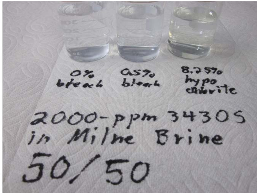
Figure 2.6: No precipitation noted when bleach was added to polymer solutions.
