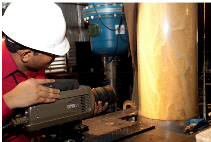
Figure 3. Researcher collecting high-speed video for particle tracking.
