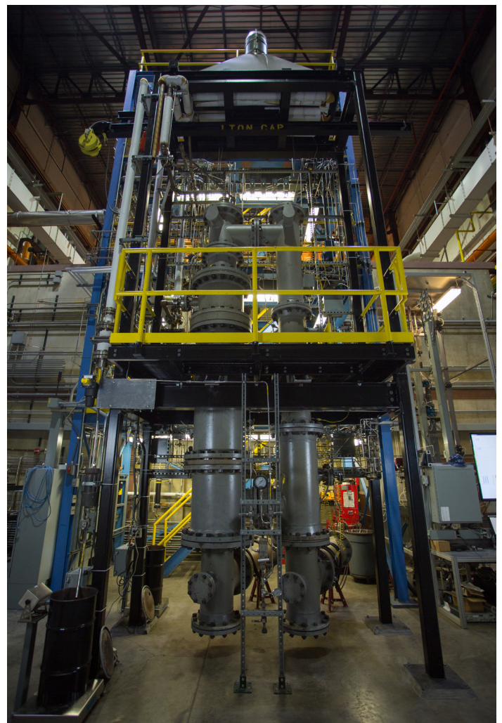
Figure 4. 50-kWth chemical looping reactor.
