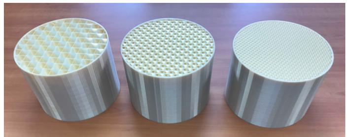
3D printed intensified packings for enhanced solvent-based CO<sub>2</sub> capture
