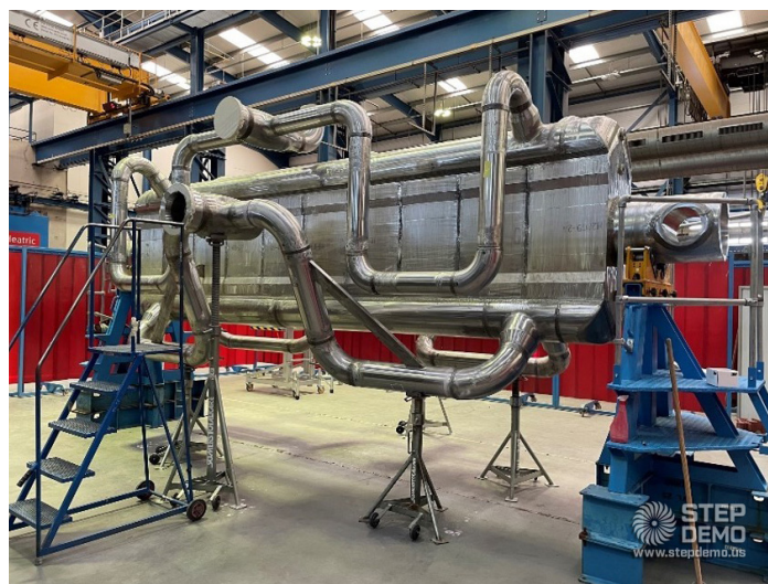
Figure 4. High Temperature Recuperator fabricated by Heatric for the 10 MWe STEP Pilot Plant Test Facility
