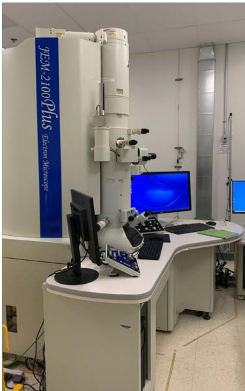
Photo 3.2.4.2: Electron Microscope at NETL Albany with specialized equipment for minerals and metals analysis.
