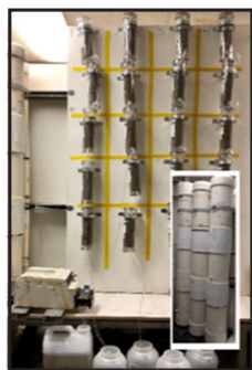
Multiple column leaching and pilot scale leaching facility (inset)
