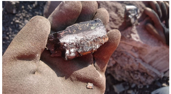
A coal sample pulled from a location within the Greater Green River and Wind River Basins of WY & CO. This sample exhibits the uniqueness of coal-based materials for CORE-CM purposes. It has high-rank coal for utility in carbon ore products as well as clay materials hosting various rare earth elements and critical minerals.
