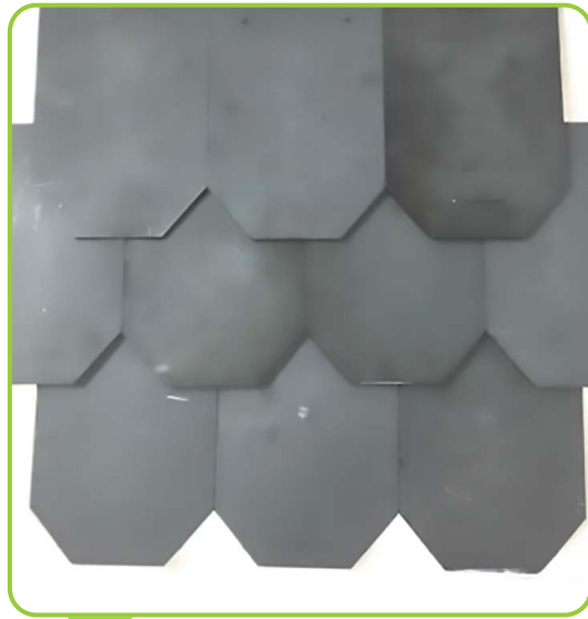
Set of 10 Coal-Based Ceramic Roof Tiles (Containing 70% Coal) Developed by Semplastics
