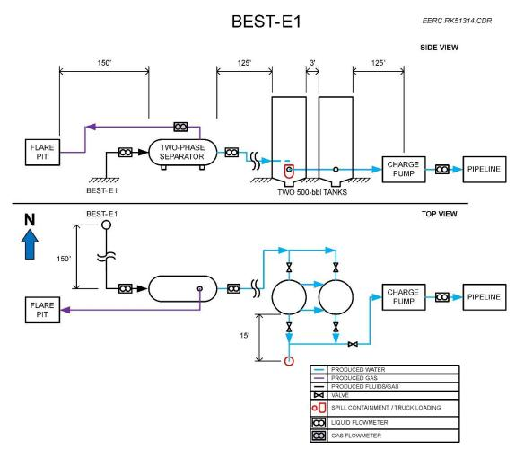
Figure 10-7. Engineering schematic of BEST-E1 facilities showing the location of major equipment and the process flow diagram between the wellhead and pipeline.
