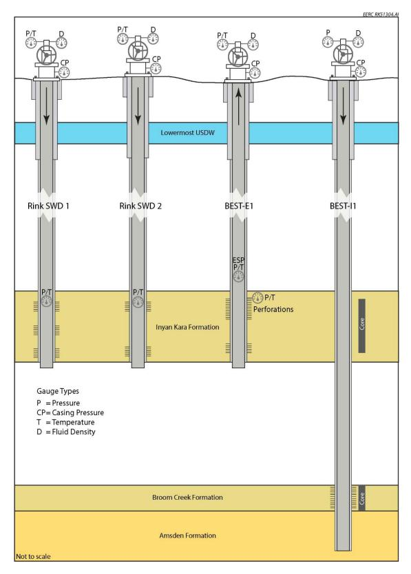
Figure 9-1. Schematic illustrating the active reservoir monitoring systems proposed for the BEST-E1, BEST-I1, Rink SWD 1, and Rink SWD 2 wells.
