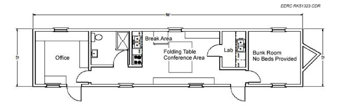
Figure D-48. Command center 12' × 56' layout design provided by contractor.
