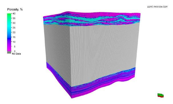
Figure A-13. Entire grid porosity property, including the Inyan Kara, Broom Creek, and Amsden Formations, as well as the interburden between the Inyan Kara and Broom Creek. The interburden was excluded from the porosity distribution (shown in gray).
