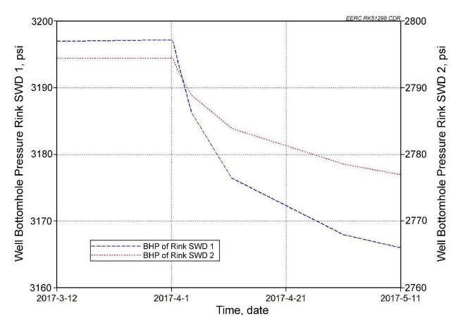
Figure A-28. Detailed bottomhole pressure response of Rink SWD 1 and Rink SWD 2, respectively, with 4000-bwpd extraction rate and 3400-bbl/day injection rate into each of the Rink SWD wells. A 10 to 20 psi pressure change is recorded within 10 days of extraction start.
