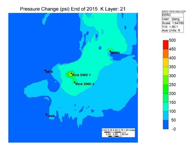
Figure A-21. Differential pressure plume distribution (psi) from year 1961 to 2015.
