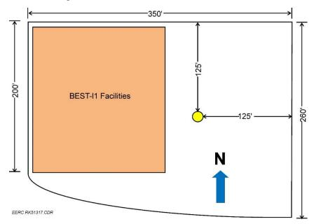
Figure D-8. Placement of facilities in relation to BEST-I1 injection well.
