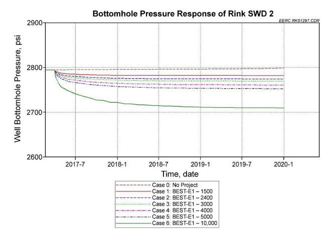
Figure 6-4. Rink SWD 2 BHP response to different extraction rates, assuming a stable 3400-bwpd injection rate into each of the Rink SWD wells.
