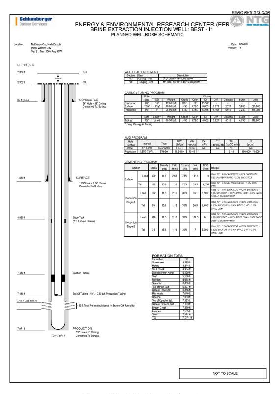
Figure 10-3. BEST-I1 well schematic.
