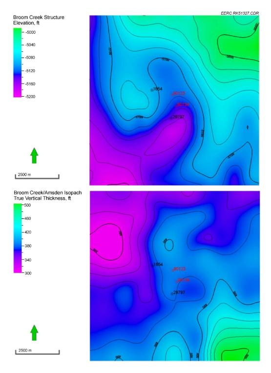
Figure A-5. Top: structure contour map on top of the Broom Creek Formation within the Johnsons Corner study area. Datum: mean sea level. Bottom: isopach map of the combined Broom Creek and Amsden Formations within the Johnsons Corner study area. Injection Wells 90123 (Rink SWD 1) and 90134 (Rink SWD 2) are shown in red. Neighboring wells that intersect the Broom Creek/Amsden are shown in black. Contour interval = 20 ft.
