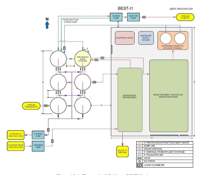
Figure 10-4. Flow path of fluids on BEST-I1 site.
