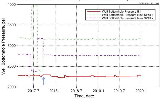
Figure 8-2. BHP response of the wells during the entire project experimental scenario. The end of interference testing and Stage 1 is indicated by the blue arrow. Changes in pressure responses of Rink SWD 1 and 2 to changing test parameters are visible throughout the experimental run.
