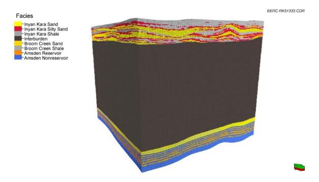
Figure A-12. Entire grid facies property, including the Inyan Kara, Broom Creek, and Amsden Formations, as well as the interburden between the Inyan Kara and Broom Creek. The interburden (shown in dark gray) was excluded from detailed facies modeling.
