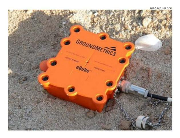
Figure A-42. Surface sensor used in borehole to surface EM surveys. An array of several hundred sensors are deployed on the surface during the survey (courtesy GroundMetrics).
