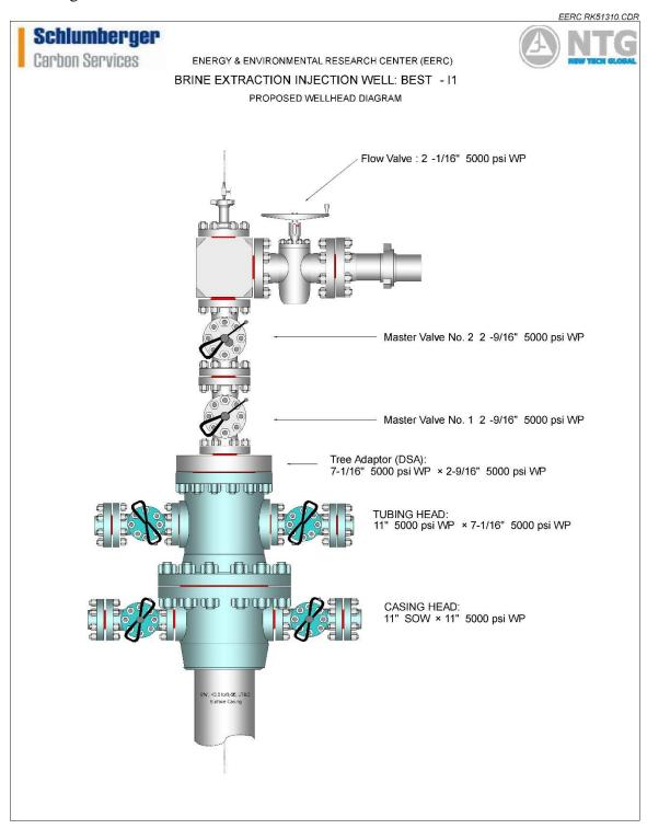
Figure D-7. BEST-I1 wellhead schematic with necessary pressure control equipment for saltwater injection provided by SLB.
