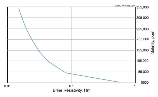
Figure A-41. Plots of brine salinity versus brine resistivity (using Crain, 1986).
