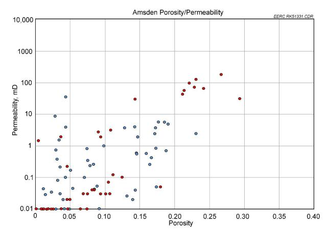
Figure A-9. Amsden porosity/permeability crossplot. This crossplot was developed from three North Dakota wells (Wells 1412, 9106, and 26249). Well 1412 (plotted in red) was approximately 3 miles from the area of interest and contained some measured permeabilities greater than 100 mD, while few values for the other two more distant wells exceeded 10 mD.
