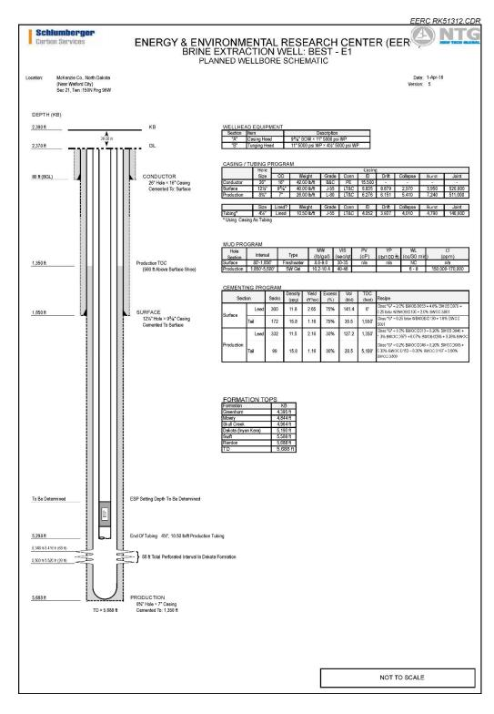
Figure 10-5. BEST-E1 well schematic.
