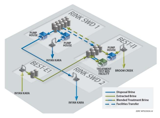
Figure 10-2. Conceptual illustration of the injection and extraction well configuration and the integrated water-handling and storage infrastructure and extracted brine treatment test bed facility.
