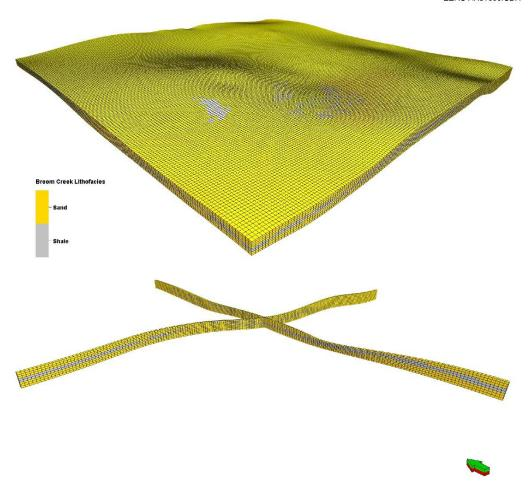
Figure 5-5. Facies distribution of the Broom Creek Formation portion of the model. The images illustrate the same full formation model view (top) and cross-section lines (bottom) as illustrated in Figure 5-4. Note that neither of the Rink SWD wells penetrates the Broom Creek, vertical exaggeration = 10×.
