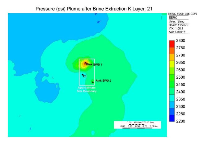
Figure A-35. Pressure (psi) plume development after Johnsons Corner project end (4000-bwpd extraction rate), showing a regional pressure decrease of 20–30 psi. Larger pressure decreases are visible near the Rink SWD 1 and 2 wells.
