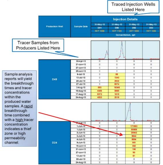
3. A final quantitative analysis report will be submitted once the survey is concluded. This will include interwell swept pore volume calculations, injected water distribution, sweep efficiency and, flow- storage capacity between wells. This report will be sent in 3-5 days after ProTechnics receives the necessary injection/ production data from the operator.
