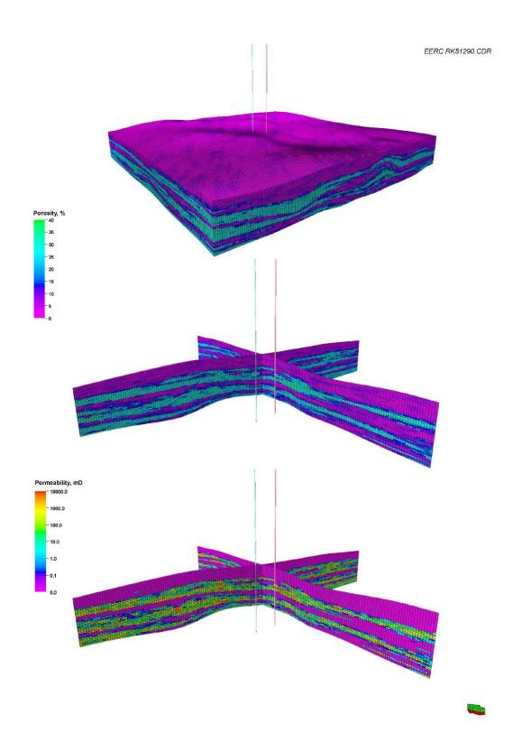
Figure 5-6. Inyan Kara Formation porosity (top) and cross sections displaying porosity (middle) and permeability (bottom). Cross sections through the model show the petrophysical properties at the two primary injection wells. The north–south trending cross section intersects Rink SWD 2 and the east–west trending cross section intersects Rink SWD 1, vertical exaggeration =  $10\times$ .
