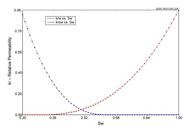
Figure A-17. Relative permeability curves used in the model.
