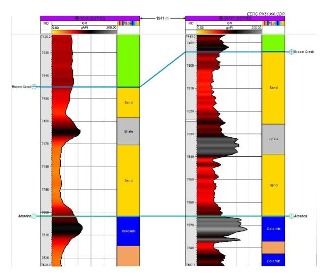
Figure 5-3. Correlation of wells 1854 (left) and 29797 (right), which are in close proximity to the Rink SWD wells (90123 and 90134). Curves shown are GR (left) and a facies log (right).
