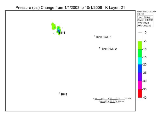
Figure A-18. Pressure difference map from January 1, 2003, to October 1, 2008, illustrating the maximum pressure differential resulting from Well 8816.
