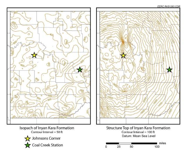
Figure 3-4. Left: isopach map of the Inyan Kara Formation in western North Dakota, contour interval = 50 feet (modified from LeFever, 2015). Isopach map shows the Inyan Kara is approximately 400 ft thick at both study sites. Right: structure contour map of the Inyan Kara Formation in western North Dakota, contour interval = 100 feet (modified from Anderson and Juenker, 2006).
