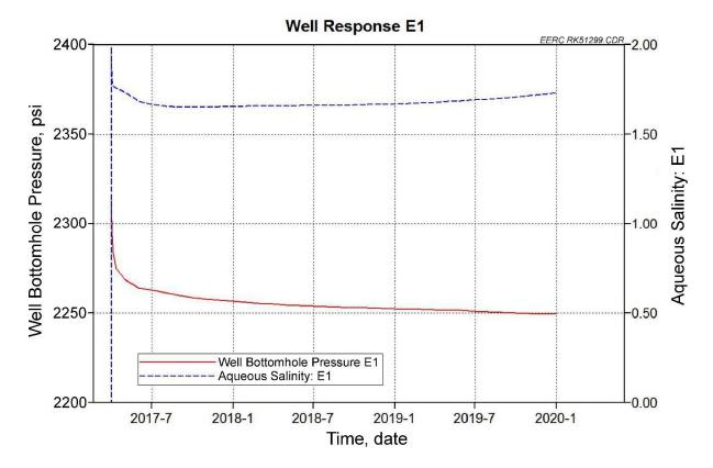
Figure 6-6. BHP and salinity changes predicted for the BEST-E1 extraction well at a 4000-bwpd extraction rate during the project lifetime. Limited pressure decline of the well is indicative of high permeability in the area.
