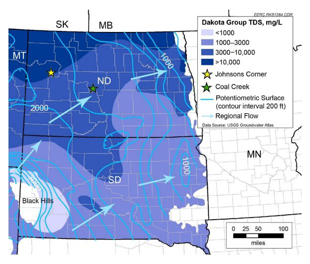
Figure 3-5. Potentiometric surface and TDS map of the Lower Cretaceous aquifers of the greater Williston Basin region, including the Inyan Kara Formation in North Dakota (adapted from Whitehead, 1996). Generalized regional flow from southwest to northeast is illustrated.
