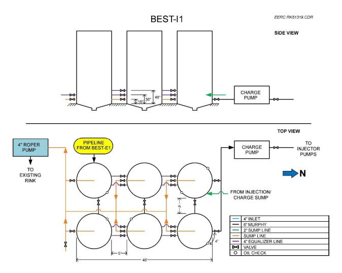
Figure D-10. BEST-I1 tank farm schematic.
