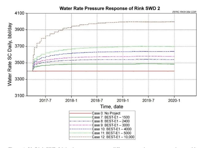
Figure A-30. Rink SWD 2 injection rate response to different extraction rates, assuming a stable wellhead pressure of 450 psi.
