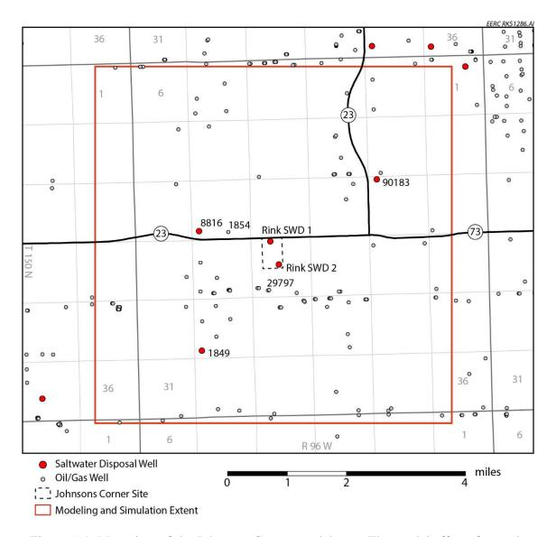
Figure 5-1. Map view of the Johnsons Corner model area. The model efforts focused on a 6-mile by 6-mile (36-mi<sup>2</sup>) area, delineated by the red rectangle.
