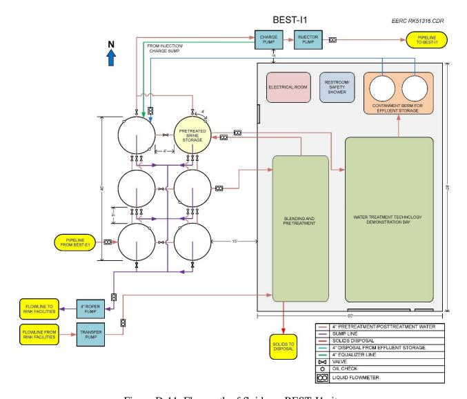
Figure D-11. Flow path of fluids on BEST-I1 site.
