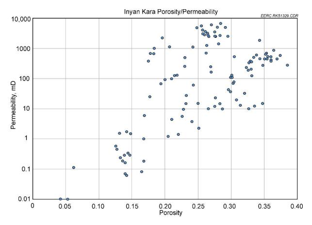
Figure A-7. Inyan Kara core porosity/permeability crossplot.
