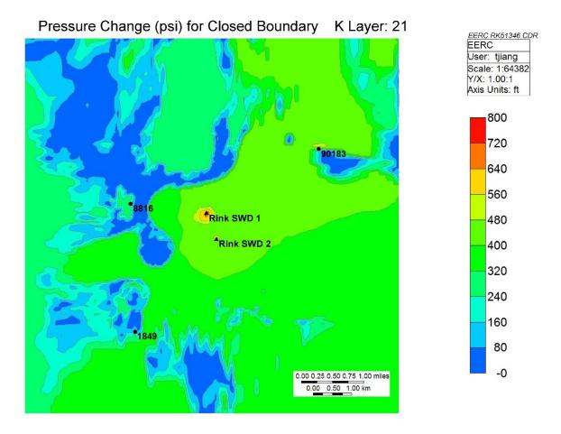
Figure A-22. Pressure buildup for the closed boundary system sensitivity case (psi).
