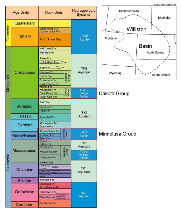
Figure 3-1. Williston Basin stratigraphic and hydrogeologic column (modified from Glazewski and others, 2015).
