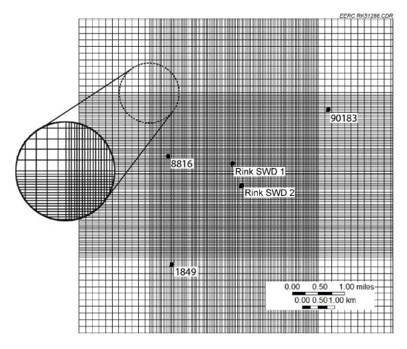
Figure 6-1. The uniform-tartan grid system configuration of the reservoir simulation model (6-mile by 6-mile area). The primary investigation area is represented by the fine uniform interior gridding.
