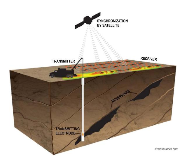
Figure A-43. Schematic from GroundMetrics, a BSEM provider, shows the survey geometry with a downhole electrode, surface transmitter, and surface receiver array synchronized by GPS satellite (courtesy GroundMetrics).
