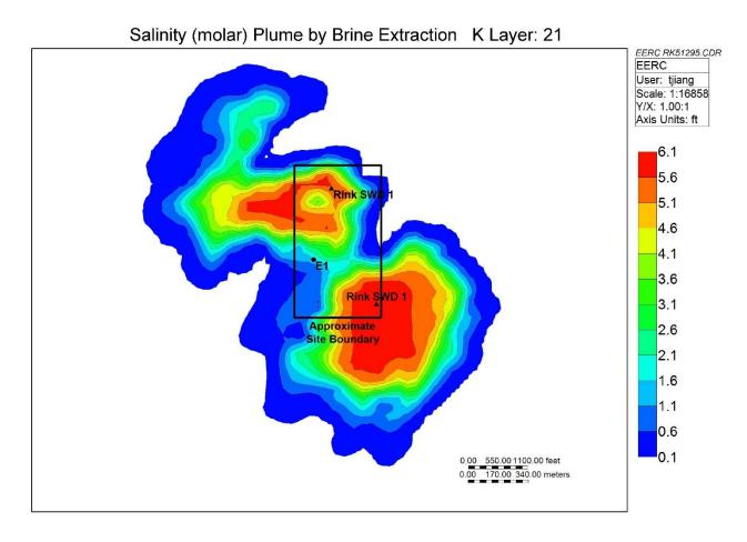
Figure A-38. Salinity (molar concentration) plume development after Johnsons Corner pilot end (4000-bwpd extraction rate). Note the significantly reduced footprint of the plume on the southwest side of the site.
