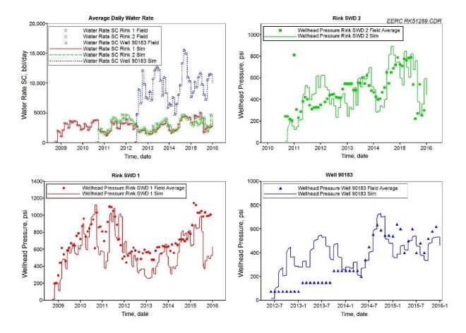
Figure 6-2. Wellhead pressure history match of Rink SWD 1 and Rink SWD 2 capture the operating trends of their injection and operating histories. Reported WHP data may be imprecise, as suggested by the early pressure history of the offset Well No. 90183.
