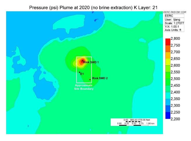
Figure A-34. Pressure (psi) plume development without the BEST project, showing an elevated pressure plume which covers the majority of the project site
