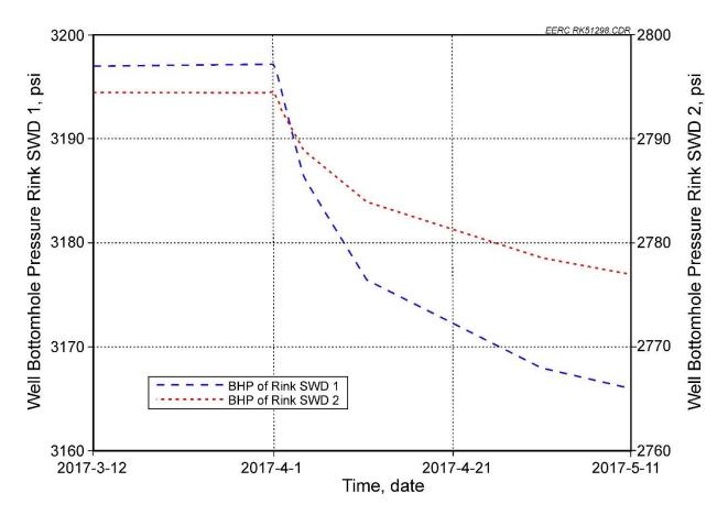
Figure 6-5. Detailed BHP response of Rink SWD 1 and SWD 2 with a 4000-bwpd extraction rate and a 3400-bwpd injection rate into each of the Rink SWD wells. A 10- to 20-psi pressure change is recorded within 10 days of extraction start.
