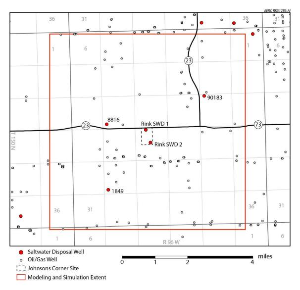
Figure A-1. Map view of the Johnsons Corner model area. The model efforts focused on a 6-mile by 6-mile (36-mi<sup>2</sup>) area (red rectangle).
