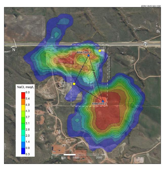
Figure 6-3. Distribution of the salinity plume on 1 April 2017 (as determined by simulation, within the Inyan Kara Formation superimposed over a site map). Proposed project wells are identified.
