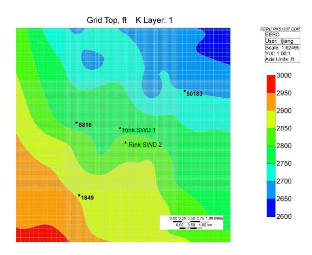
Figure A-16. The reservoir simulation model with a uniform-tartan grid system superimposed on the Inyan Kara top structure map (6 miles by 6 miles).
