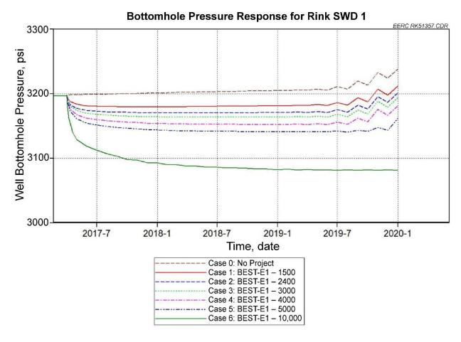
Figure A-26. Rink SWD 1 bottomhole pressure response to different extraction rates, assuming a stable 3400-bbl/day injection rate into each of the Rink SWD wells.
