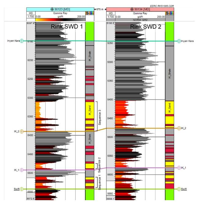
Figure 5-2. Correlation of injection wells Rink SWD 1 (left) and Rink SWD 2 (right). Curves shown for each well are GR and a facies log. The Inyan Kara Formation is split into three fining upward sequences.
