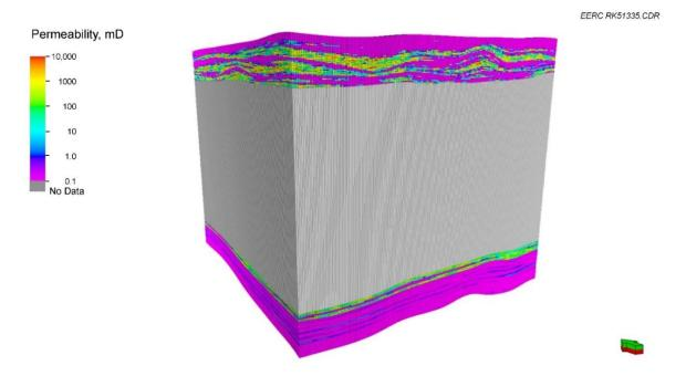
Figure A-14. Entire grid permeability property, including the Inyan Kara, Broom Creek, and Amsden Formations, as well as the interburden between the Inyan Kara and Broom Creek. The interburden was excluded from the permeability distribution (shown in gray).
