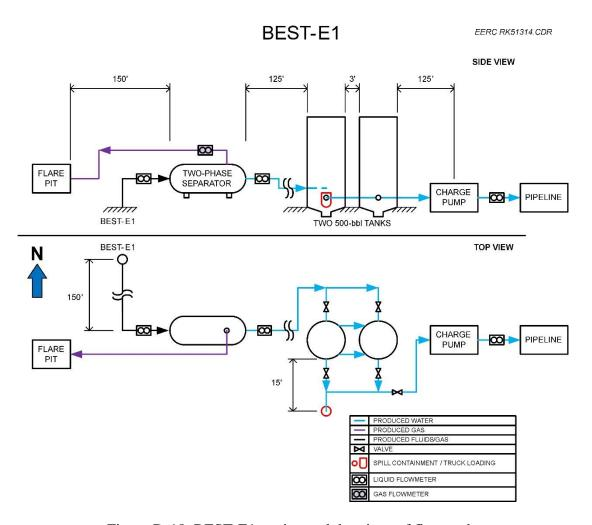
Figure D-18. BEST-E1 engineered drawings of flow path.
