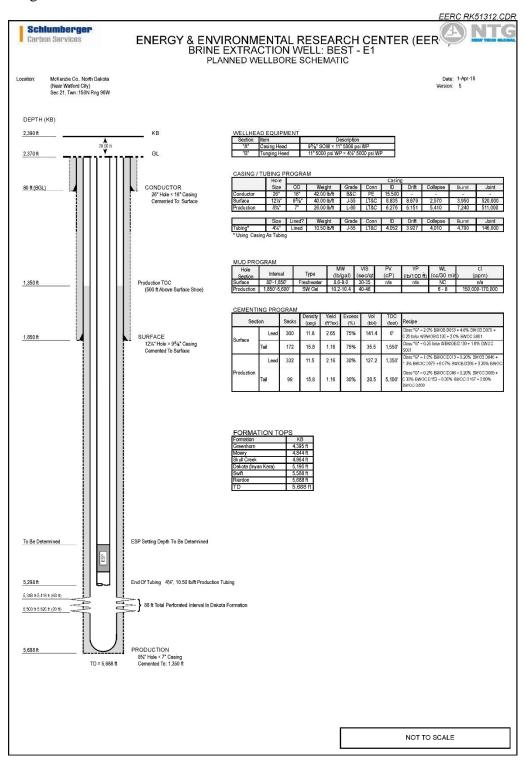
Figure D-13. Well schematic provided by SLB.
