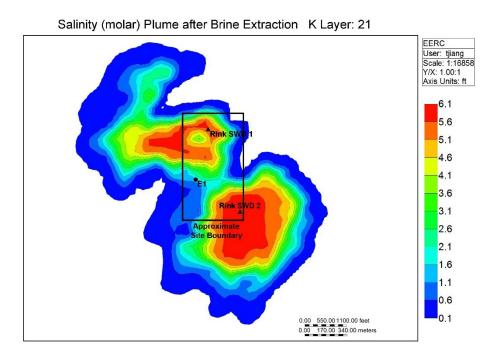
Figure 8-5. Salinity (molar concentration) of plume development in January 2020 without brine extraction, business as usual (above), and with the extraction experimental scenario (below). Note the significantly reduced footprint of the plume on the southwest side of the site.
