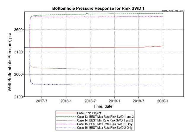
Figure A-31. Bottomhole pressure response of Rink SWD 1 for Cases 13 through 16.
