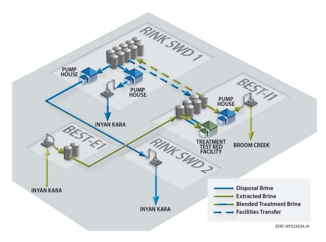
Figure 1-1. Conceptual illustration of the injection and extraction well configuration and the integrated water-handling and storage infrastructure and extracted brine treatment test bed facility.
