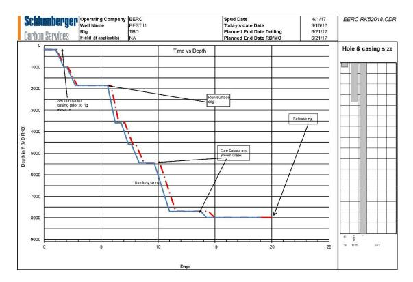
Figure D-1. Proposed time line for BEST-I1 well drilling provided by SLB.
