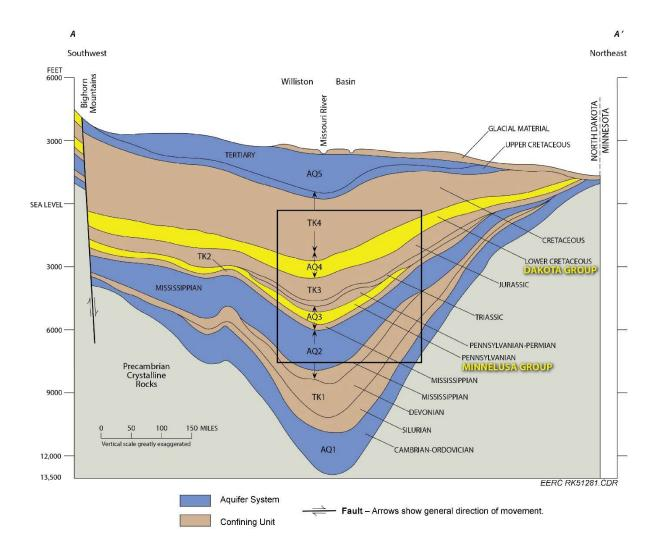
Figure 3-2. A cross section of the Williston Basin illustrating the five major aquifer systems. The Dakota and Minnelusa Groups are highlighted in yellow (modified from Downey and others, 1987). The portion of the basin evaluated is highlighted by the box.
