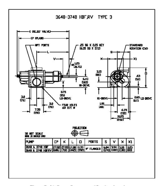
Figure D-31. Roper Pumps specification data sheet.
