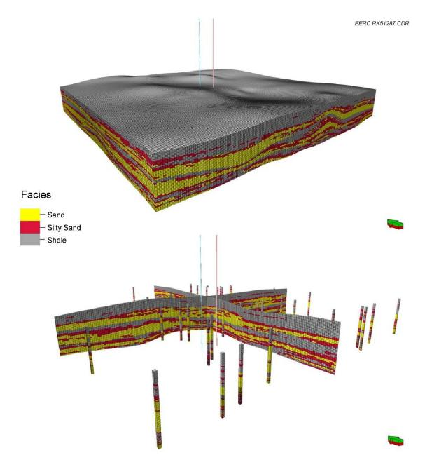
Figure 5-4. Facies distribution in the Inyan Kara Formation model. Top image illustrates the full Inyan Kara Formation model. Bottom image shows cross sections running through Rink SWD 2 in the north–south direction and Rink SWD 1 in the east–west direction, as well as the interspersed control points used to guide the MPS distribution, vertical exaggeration =  $10\times$ .
