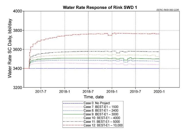
Figure A-29. Rink SWD 1 injection rate response to different extraction rates, assuming a stable wellhead pressure of 958 psi.
