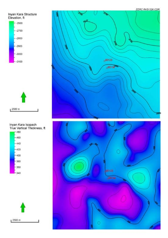
Figure A-4. Top: structure contour map on top of the Inyan Kara Formation within the Johnsons Corner study area. Datum: mean sea level. Bottom: isopach map of the Inyan Kara Formation within the Johnsons Corner study area. Injection Wells 90123 (Rink SWD 1) and 90134 (Rink SWD 2) are shown in red. Contour interval = 20 ft.
