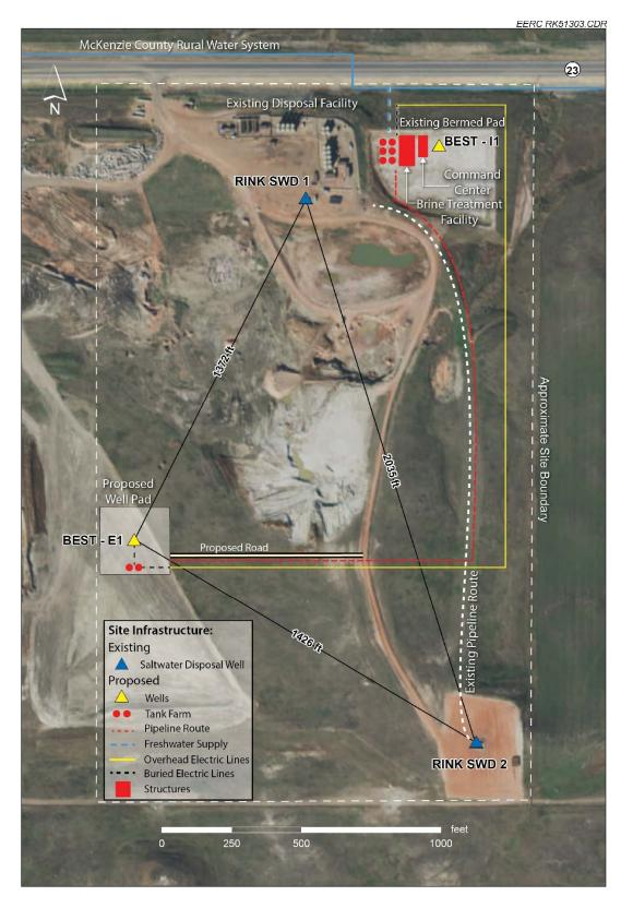
Figure A-25. Selected well locations for Johnsons Corner project execution and placement of associated new infrastructure.
