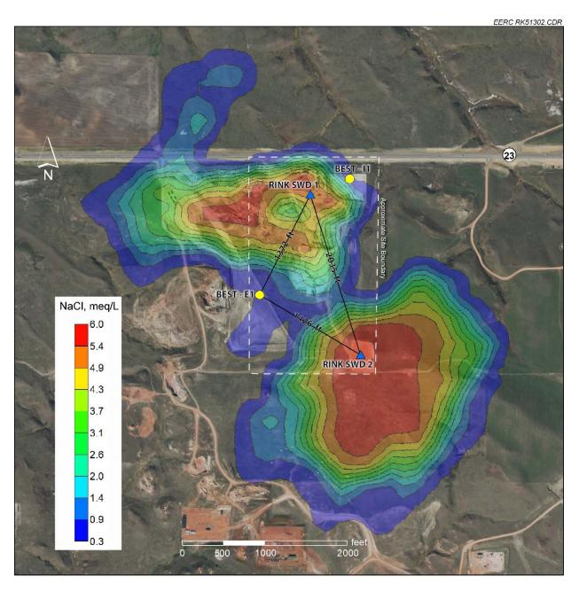
Figure A-23. Interpreted salinity distribution within the Inyan Kara Formation on 1 April 2017 superimposed over a site map. Salinity scale is NaCl molarity. Existing and proposed project wells are named.
