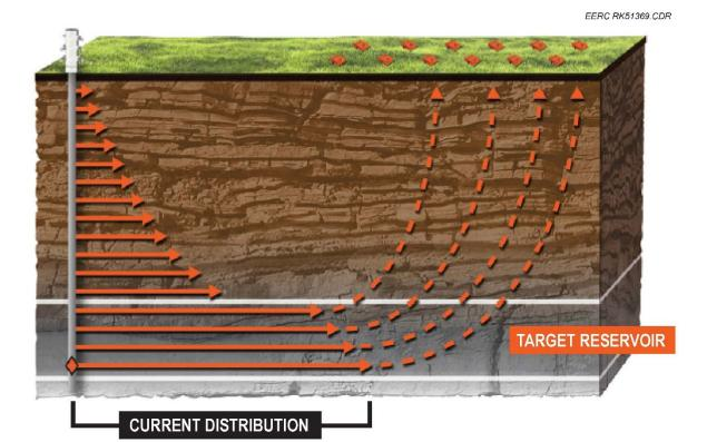
Figure A-44. Schematic of injected current moving through the target reservoir and returning to the surface where it is detected by the sensors (courtesy GroundMetrics).
