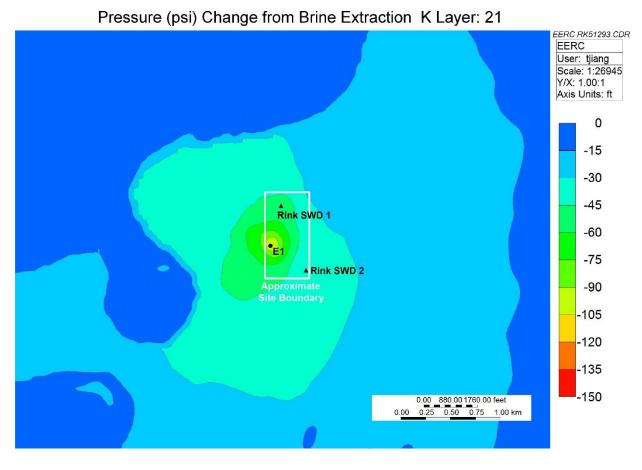
Figure A-36. Pressure (psi) difference map illustrating the influence of the extraction scenario in the year 2020.
