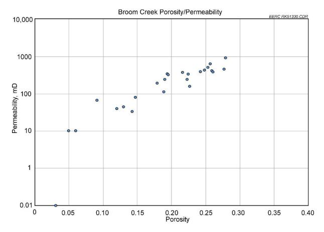
Figure A-8. Broom Creek porosity/permeability crossplot.
