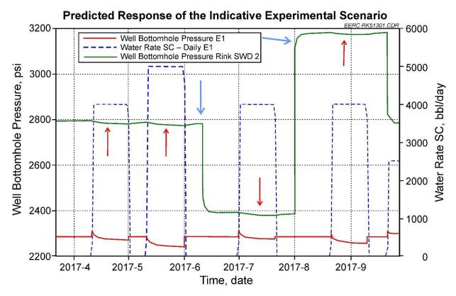
Figure 8-1. Predicted pressure response of the Rink SWD 2 well to changes in extraction rate. Changes in BHP due to changing injection rates are clearly visible (indicated by blue arrows). However, subtle dips in the BHP of Rink SWD 2 also occur in response to fluid extraction from the BEST-E1 well (indicated by red arrows).
