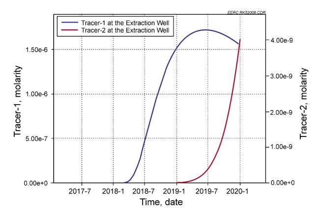
Figure 8-7. Tracer response at the BEST-E1 extraction well. Time of tracer injection is May 2017. Tracer 1 is injected into the Rink SWD 1; tracer 2 is injected into the Rink SWD 2 well.
