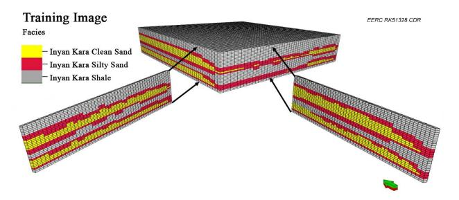
Figure A-6. Training image grid used in MPS facies distribution. Clean sand is yellow, silty sand is red, and shale is gray. Cross sections in the X and Y direction show the internal structure of the training image.
