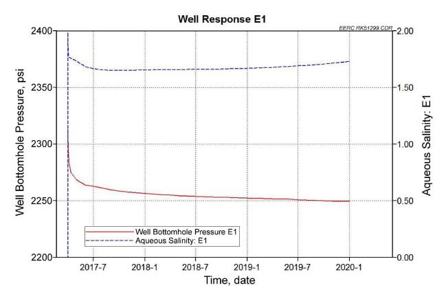
Figure A-33. Bottomhole pressure and salinity performance of the BEST-E1 extraction well.
