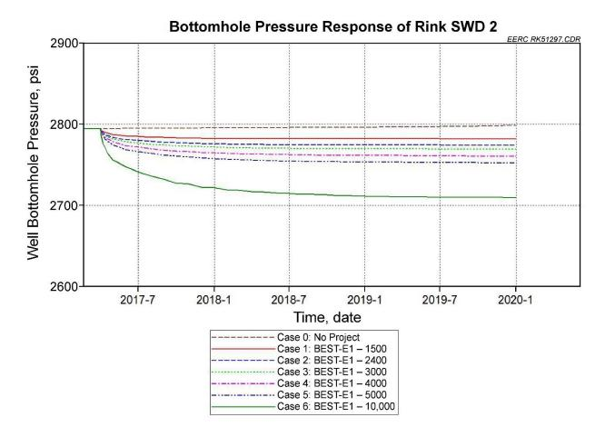
Figure A-27. Rink SWD 2 bottomhole pressure response to different extraction rates, assuming a stable 3400-bbl/day injection rate into each of the Rink SWD wells.
