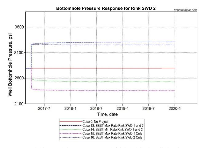
Figure A-32. Bottomhole pressure response of Rink SWD 2 for Cases 13 through 16.
