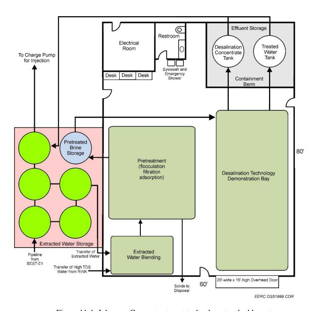
Figure 11-1. Johnsons Corner treatment technology test bed layout.
