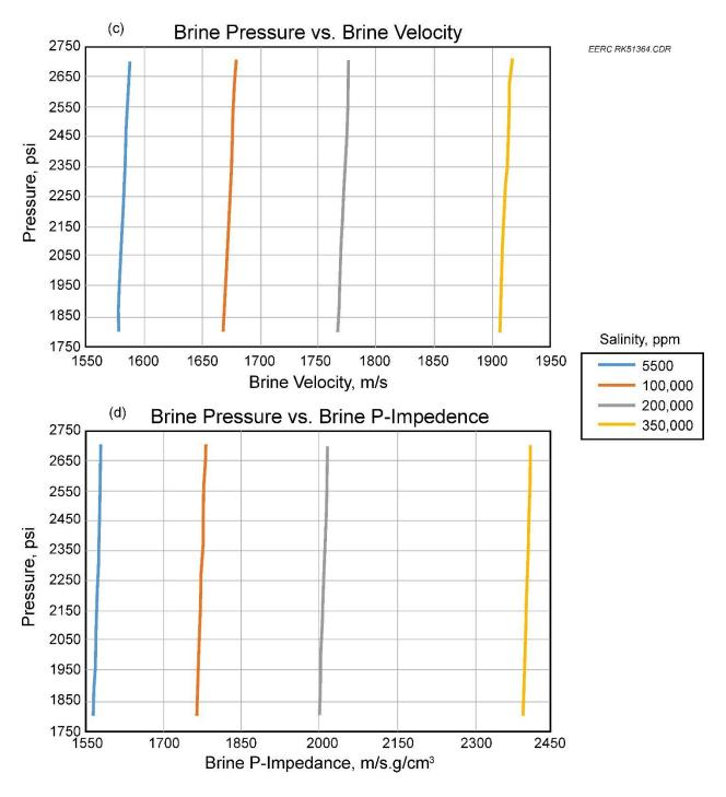
Figure A-40. Plots of pressure versus a) brine density, b) brine bulk modulus, c) brine velocity, and d) brine P-impedance at an average reservoir temperature of 135°F for different salinities as indicated (using Han and Batzle, 2002).
