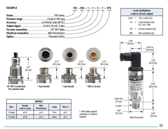
Figure D-47. NOSHOK-provided 100 Series pressure sensor transmitters and transducers specification data sheet (page 2).
