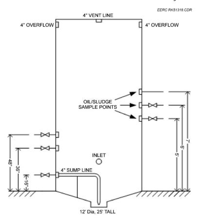
Figure D-9. Individual 500-bbl fiberglass tank schematic.
