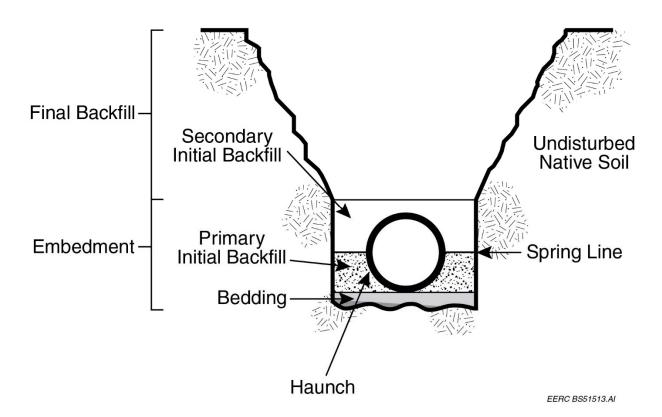
Figure D-22. Cross section of pipeline trench and backfill stages (Plastic Pipes Institute, 2009).
