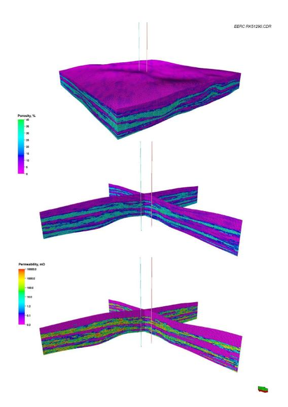
Figure A-10. Inyan Kara Formation porosity (top) and cross sections displaying porosity (middle) and permeability (bottom). Cross sections through the model show the petrophysical properties at the two primary injection wells. The north–south trending cross section intersects Rink SWD 2, and the east–west trending cross section intersects Rink SWD 1. Vertical exaggeration =  $10\times$ .
