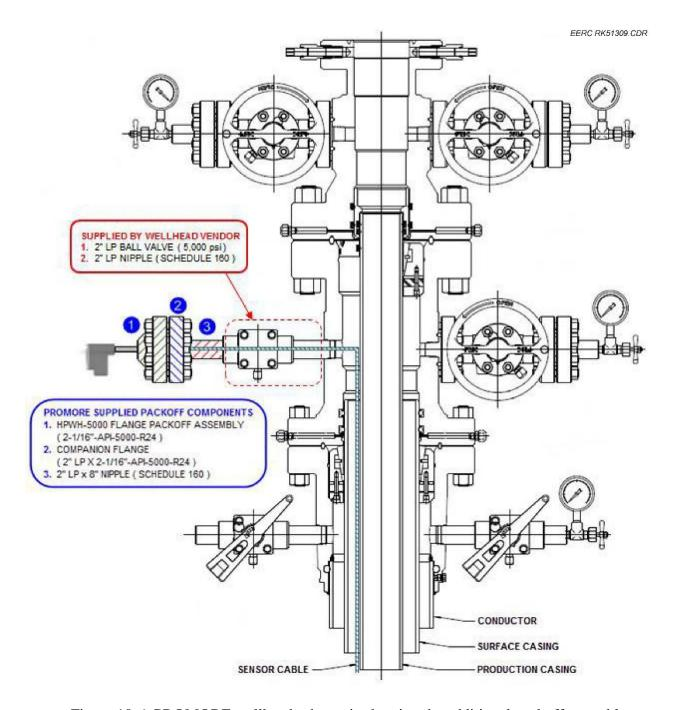
Figure 10-6. PROMORE wellhead schematic showing the additional packoff assembly necessary for installation of the downhole instrumentation.
