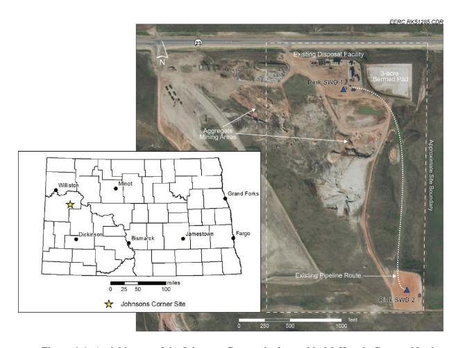
Figure 4-1. Aerial image of the Johnsons Corner site located in McKenzie County, North Dakota, highlighting the location of existing mining, lease roads, brine-handling facilities, pipeline, prepared pad for permitted extracted brine treatment facilities, and the existing Rink SWD 1 and Rink SWD 2 wells.
