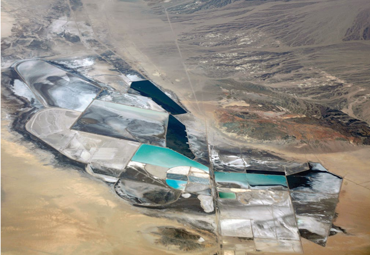
Lithium-brine evaporating ponds at Clayton Valley, Nevada. Li concentrates from 160ppm to 5,000ppm in 2 years 1
