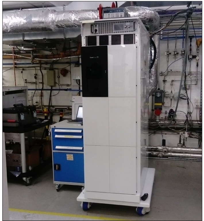
FIGURE 3. Cummins/Ceres Power 10 kW SOFC System. Photo courtesy of Cummins/Ceres Power
