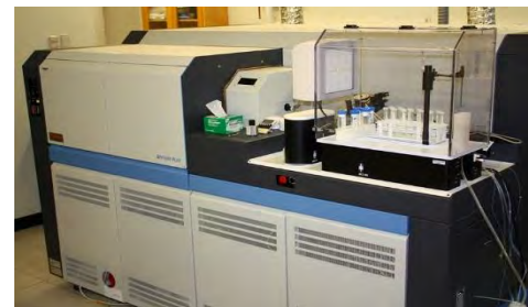
Thermo Scientific Neptune Plus MC-ICP-MS for groundwater isotopes
