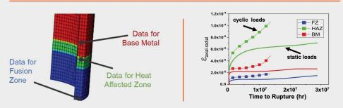
Using LaRomance (Los Alamos Reduced Order Models for Advanced Nonlinear Constitutive Equations), a surrogate model was developed for embedding into commercial finite element packages and can account for cyclical loading (demonstrated above for an idealized weld).
