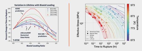
As demonstrated above for alloy P91, a rupture life criterion that considers uncertainty and is applicable to multi-axial loading was derived using limited experimental data.
