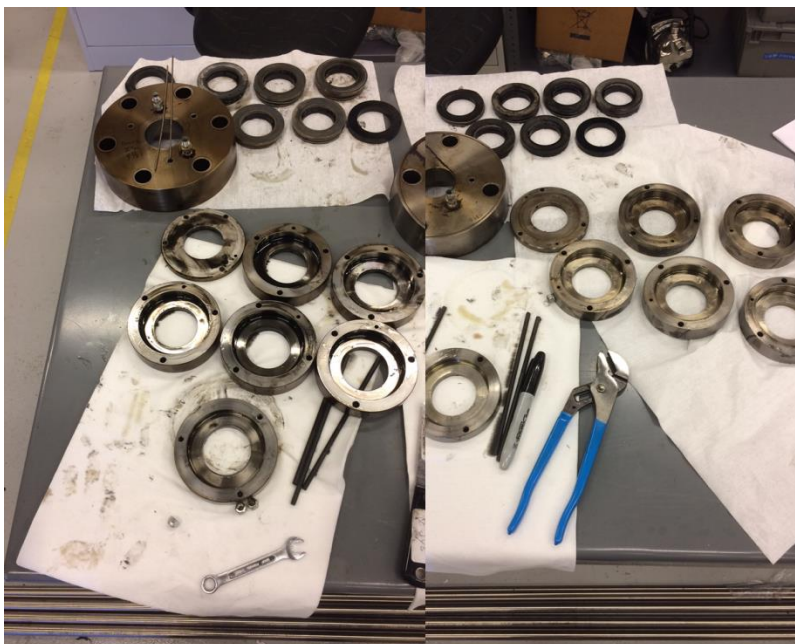
Figure 12. Torn Down Packings with Baseline Left and Used Right
