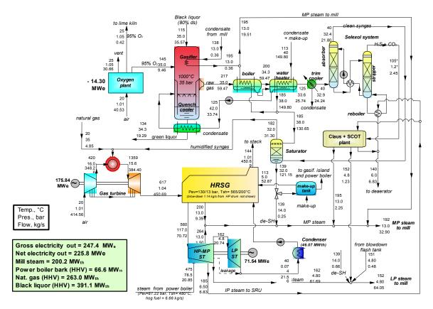
Figure S8. Energy/mass balance for BLGCC with high-temperature gasifier and utility-scale gas turbine.
