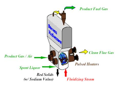
Figure 8. TRI black liquor gasification concept.
