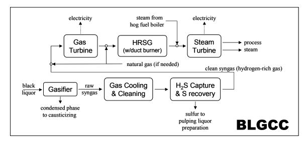
Figure 11. Simplified representation of power/recovery systems simulated in this study.
