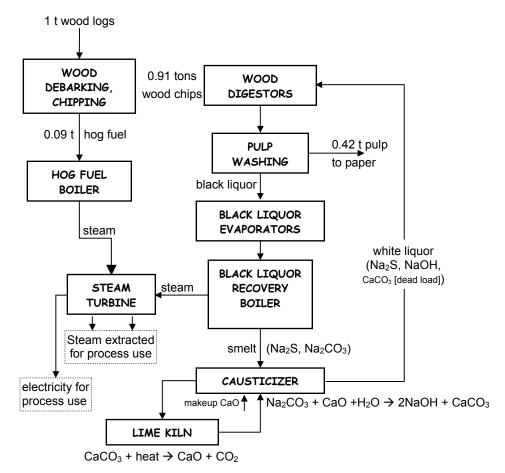
Figure S3. Simplified representation of kraft pulping and the associated chemical recovery cycle. Indicated mass balance is on a dry-matter basis and intended only to be illustrative.
