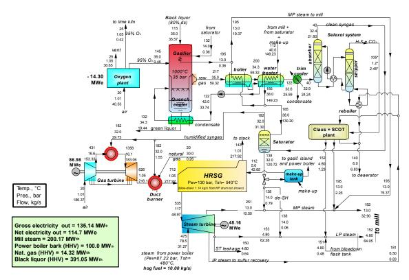
Figure S7. Energy/mass balance for BLGCC with high-temperature gasifier and mill-scale gas turbine.
