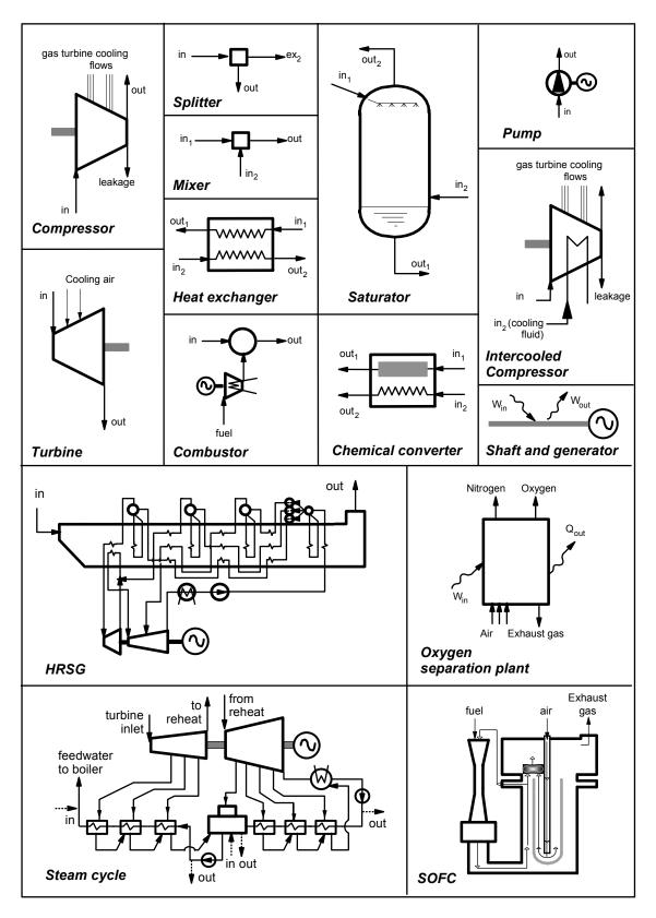
Figure A1. Components handled by the GS code.
