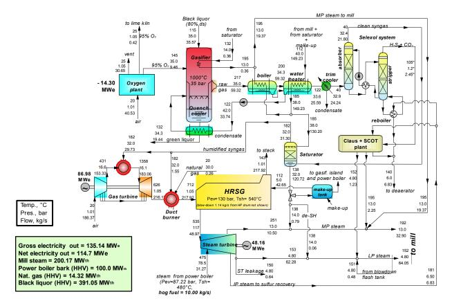
Figure 13. Energy/mass balance for BLGCC with high-temperature gasifier and mill-scale gas turbine.
