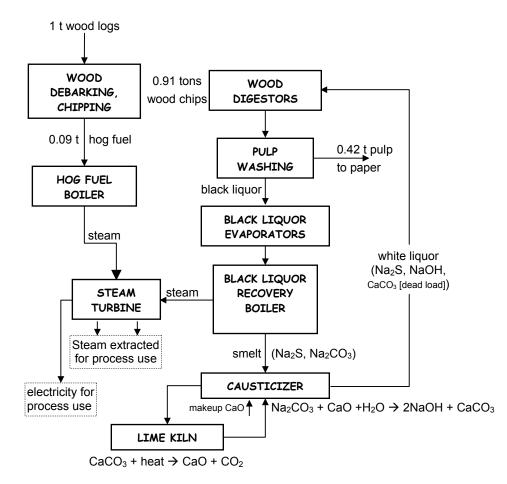
Figure 6. Simplified representation of kraft pulping and the associated chemical recovery cycle. Indicated mass flows are on a dry-matter basis and intended only to be illustrative.
