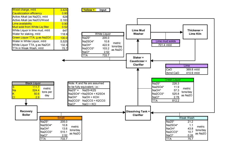
Figure A2. Estimate of causticization load for the Tomlinson base case. TTA = Total Titratable Alkali.
