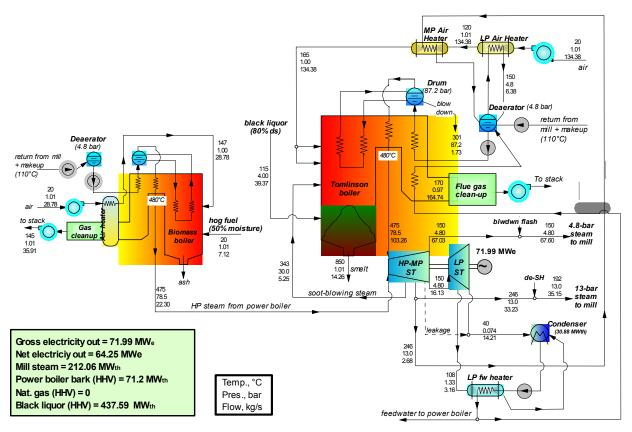
Figure 9. Energy/mass balance for the Tomlinson BASE recovery boiler.
