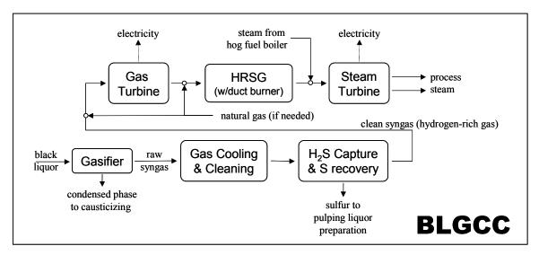
Figure S5. Simplified representation of power/recovery systems simulated in this study.
