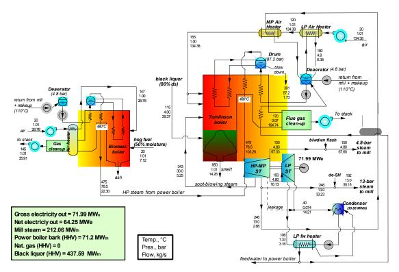
Figure S4. Energy/mass balance for Base Tomlinson recovery boiler.
