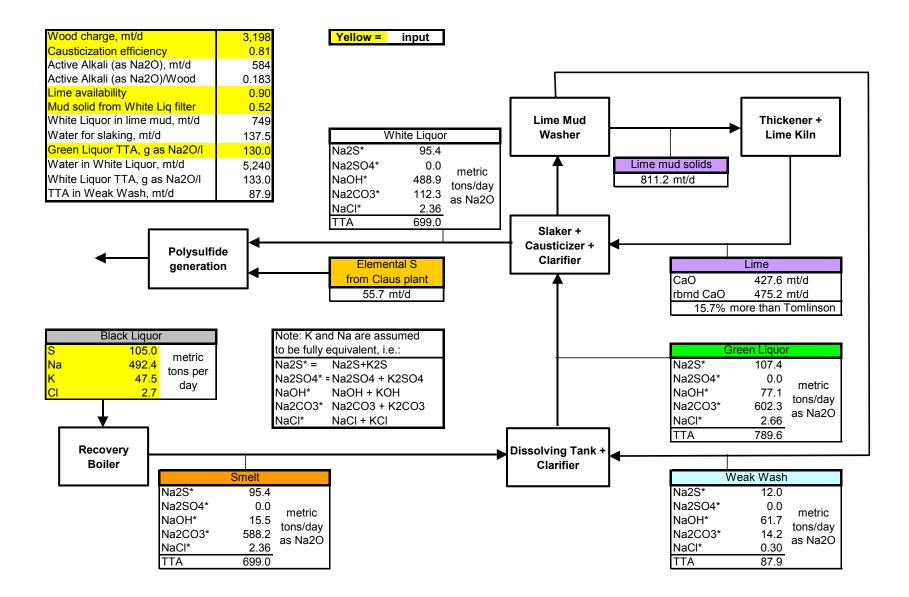
Figure A3. Estimate of causticization load for the high-temperature gasification case. TTA = Total Titratable Alkali.
