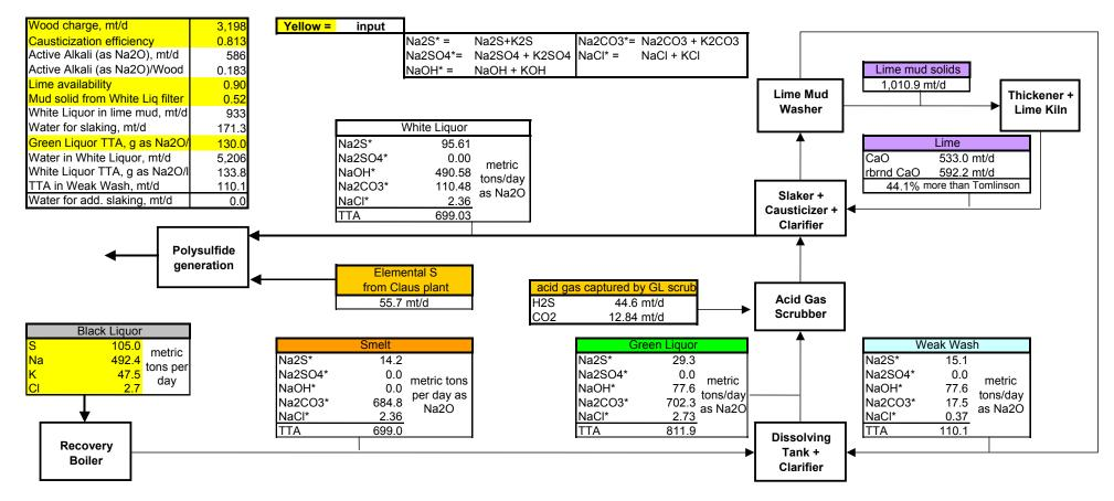
Figure A4. Estimate of causticization load for the low-temperature gasification case. TTA = Total Titratable Alkali.
