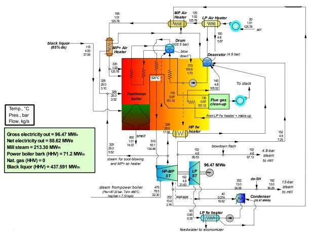
Figure 10. Energy/mass balance for high-efficiency Tomlinson recovery boiler (HERB).
