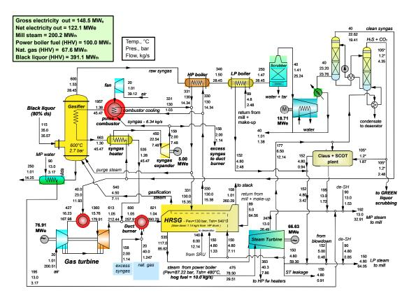
Figure 12. Energy/mass balance for BLGCC with low-temperature gasifier and mill-scale gas turbine.
