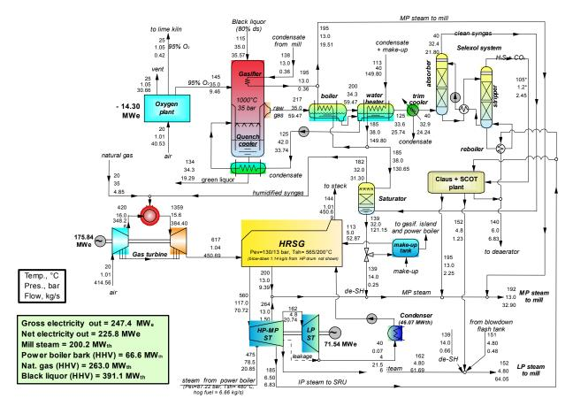
Figure 14. Energy/mass balance for BLGCC with high-temperature gasifier and utility-scale gas turbine.
