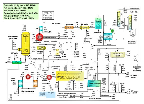
Figure S6. Energy/mass balance for BLGCC with low-temperature gasifier and mill-scale gas turbine.
