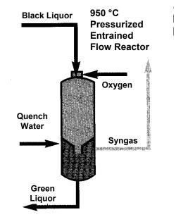
Figure 7. Chemrec black liquor gasification concept.
