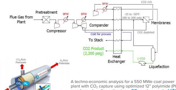
plant with  $CO_2$  capture using optimized 12" polyimide (PI-2) membrane bundles estimates a CO<sub>2</sub> capture cost of "\$32/ tonne, making progress toward the DOE's capture cost target.
