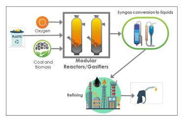
FIGURE 5. A Gasification Production Key Technology— Coal & Biomass to Liquids and Polygeneration
