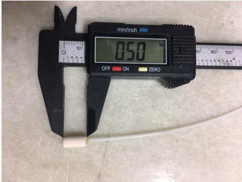
**Fig. 2.14. Porous ceramic capillary pressure sensor.**
