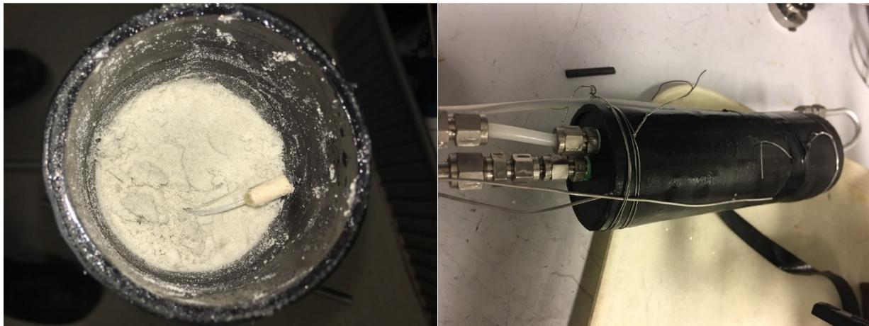
**Fig.2.15. (a) . Packing sensor and sand inside elastomer sleeve. (b) Packed elastomer sleeve, showing inlet end cap with two inlets, a central one for fluid flow and temperature measurement, the other to accommodate the three capillary sensors.**
