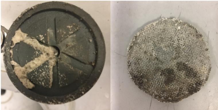
**Fig. 2.10. Outlet endcap and screen after disassembly showing some sand migration through the screen.**
