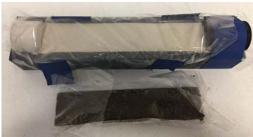
**Fig. 2.3. Layered sample preparation. Top - sand in half-cylinder mold, middle - mud sample, bottom - both. Plastic wrap was used to protect sample and prevent evaporation during freezing.**
