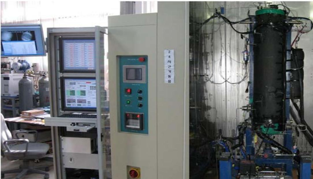
**Fig. 1.4** Picture of the experimental setup for 1D 1-m scale GH production (KIGAM 2011)
