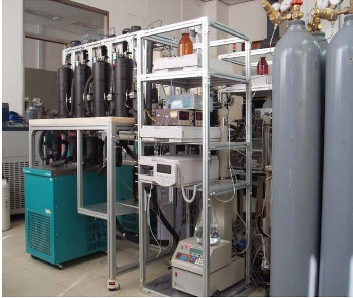
**Fig. 1.2 Permeability measurement system of hydrate-bearing sediments (1. Sand column 2. Heise Transducer, 3. Differential Pressure Transducer, 4. Back Pressure Regulator, 5. Mass Flow Meter, 6. Mass Flow Controller, 7. Reciprocating Pump, 8. CH<sub>4</sub> Cylinder, 9. Syringe Pump, 10. Displacement gauge, Red Rectangles: Temperature controlled unit) (KIGAM 2007)**
