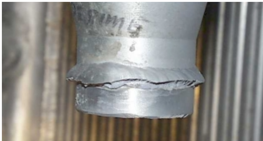
Figure 5.1.4D: Derime Header Failed Weld
