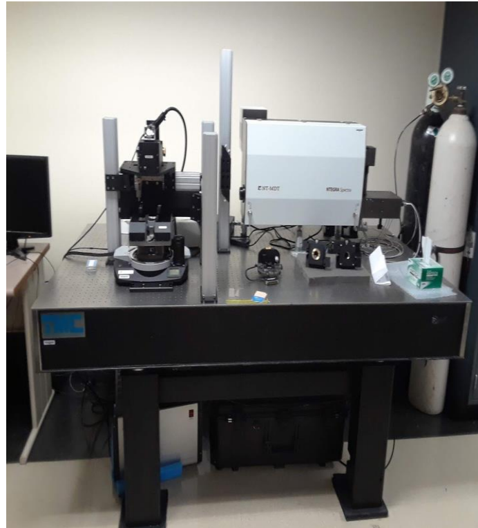
Integrated setup for SPM and Raman characterization
