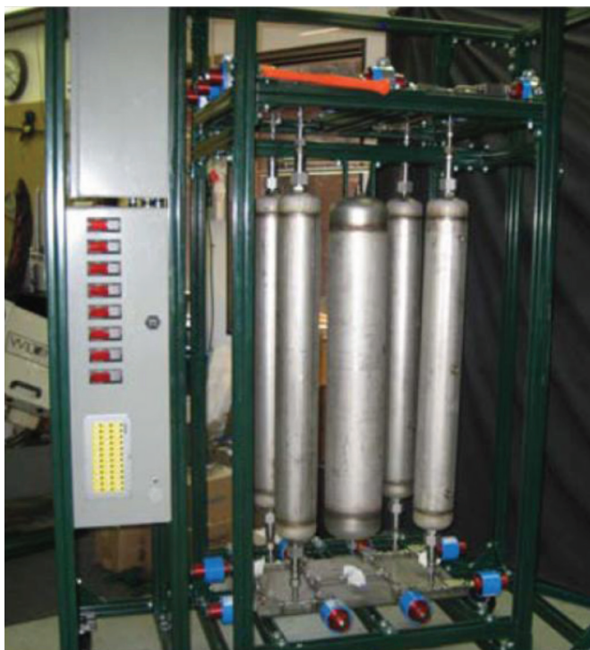
TDA's Carbon-Based Sorbent Slipstream Test Skid at NCCC
