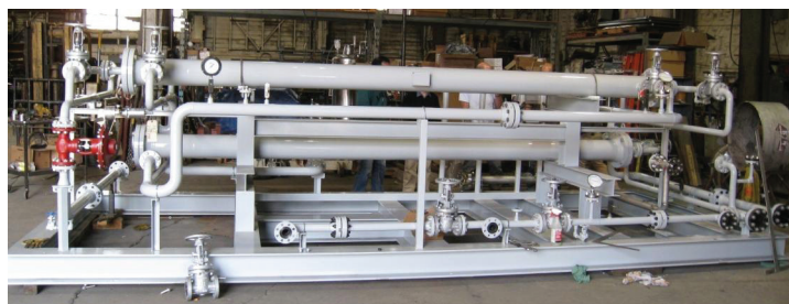
MTR's 0.05 MW Membrane Test Skid
