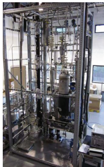
ION Engineering's Ionic Liquid Bench-Scale Test Equipment
