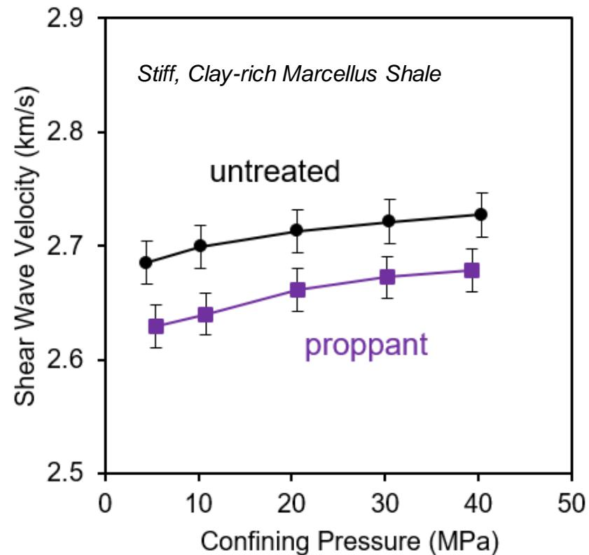
Stiff, clay-rich formation: producing (propped) fractures can be seismically detected!
