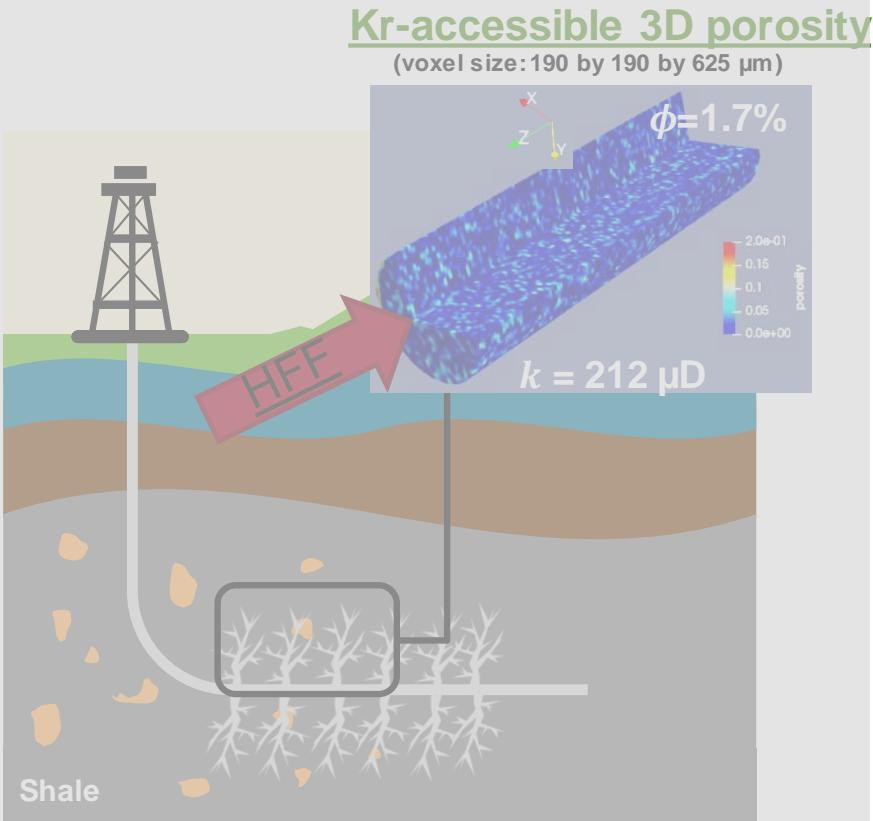
**The solution:** Manipulate chemistry and injection pressure to promote an altered zone.
