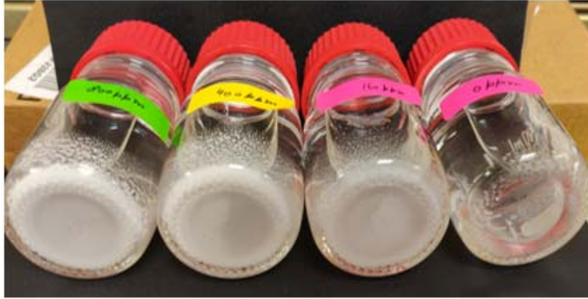
Figure 6.15: Cloud point test solutions after 24 hours at 250°F.
