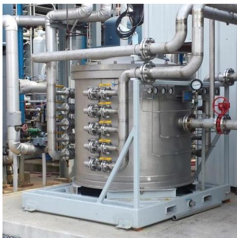
Figure 8: Prototype plate-and-frame module during testing at NCCC.
