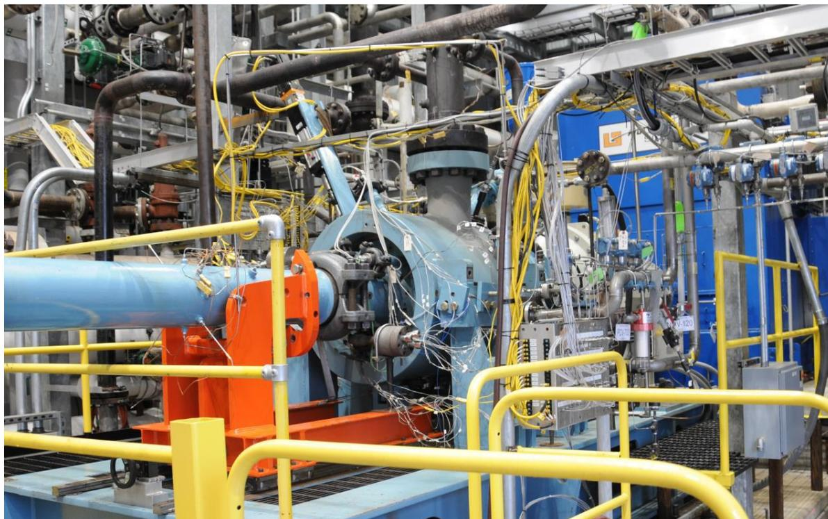
Figure 3: High-pressure CO<sub>2</sub> compressor on test stand.
