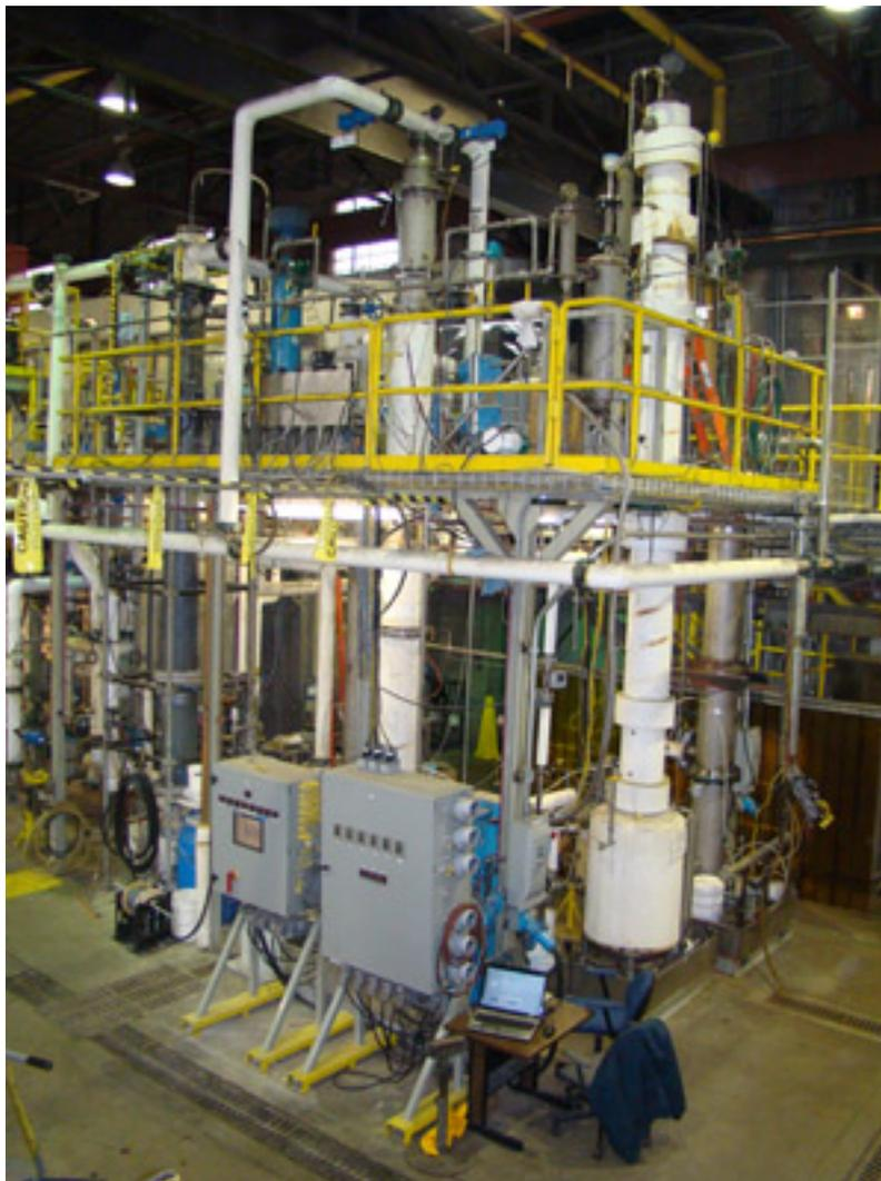
Figure 1: UNDEERC post-combustion CO<sub>2</sub> capture test facility
