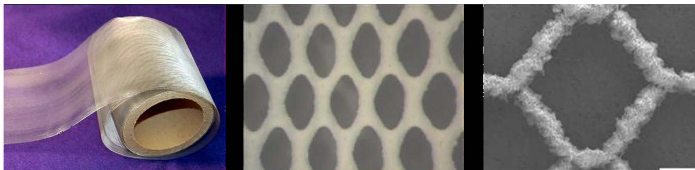
Figure 1: Microlith® mesh coated with sorbent.
