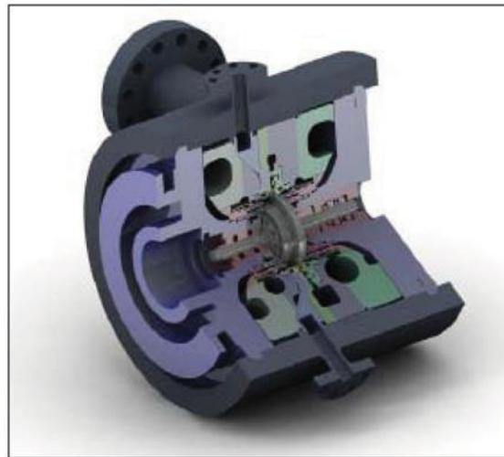
Figure 1: Cross-sectional model of a single-stage supersonic compressor.
