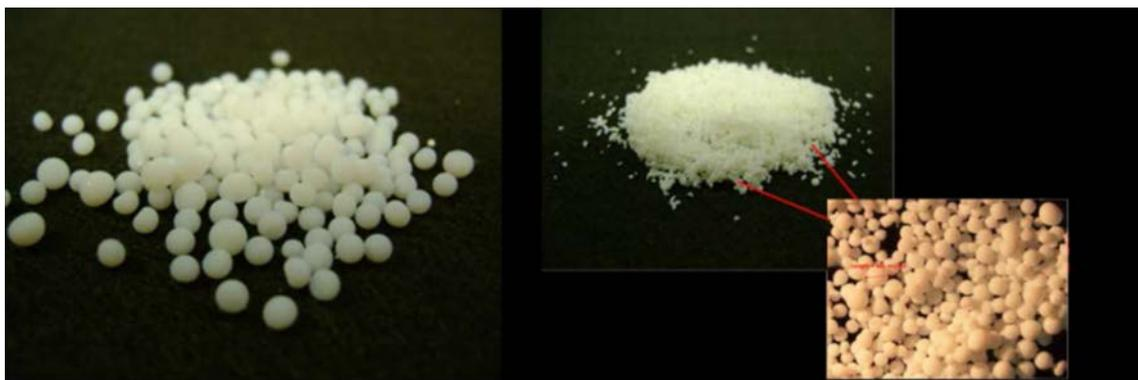
Figure 2: AFA sorbent in bead form
