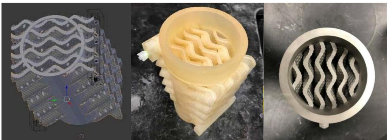
Figure 3: 3D-printed packing.
