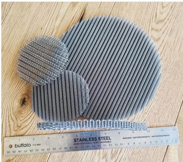
Figure 2: Froth generating and propagation screens.
