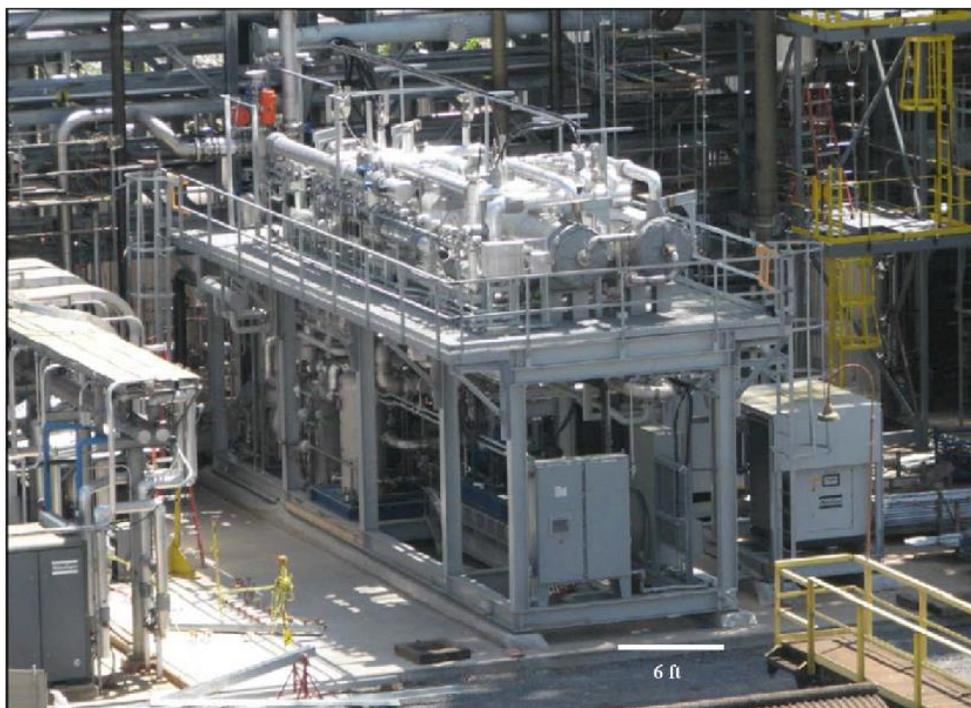
Figure 6: 20-TPD small pilot system installed at NCCC.
