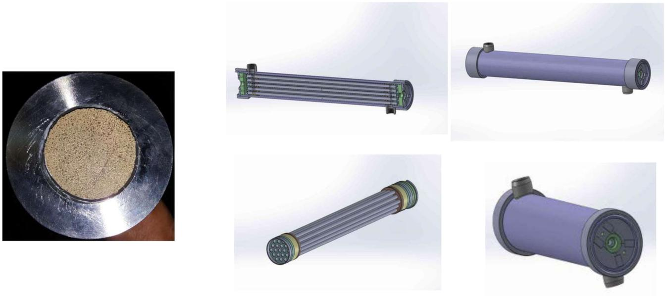
Figure 4: Potted module cross-section (left-most); new tube sheet module design (right).
