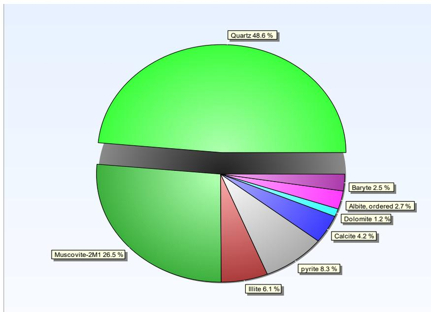
Figure 3.4c MSEEL Rietveld quantification of target formation as a pie chart, showing mineral composition in weight percent.
