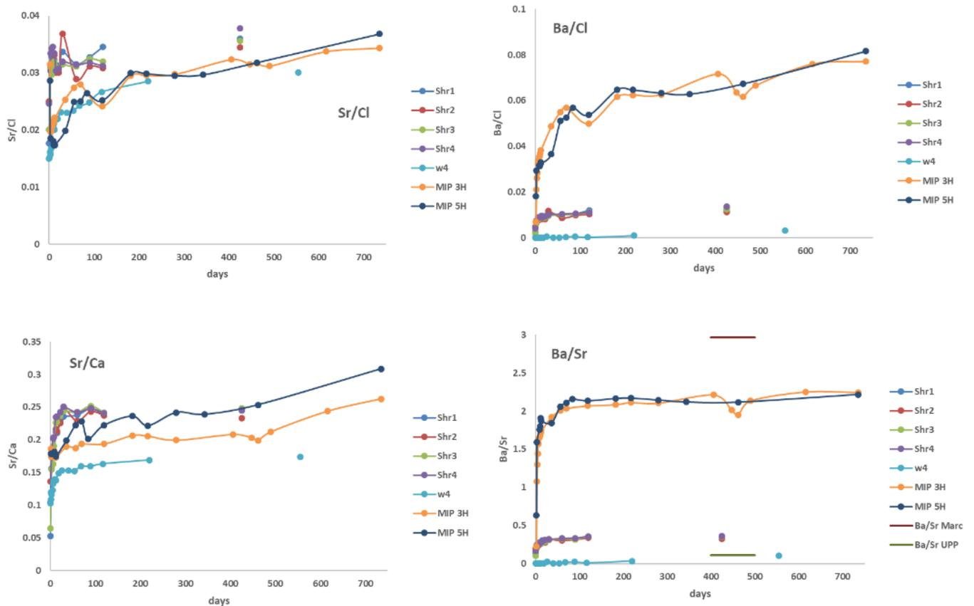
**Figure 3.2 Elemental ratios for UPP and MSEEL fluids (wt:wt ratios). Top left Sr/Cl, bottom left Sr/Ca, top right Ba/Cl and bottom right Ba/Sr in flowback fluids from MSEEL and UPP wells showing an increase in the Ba/Cl and Sr/Cl ratios over time. The increase in alkaline earth elements compared to Cl reflects ion exchange reactions and dissolution of Sr and Ba bearing phases such as barite/celestite or gypsum, carbonates, or phosphate minerals.**
