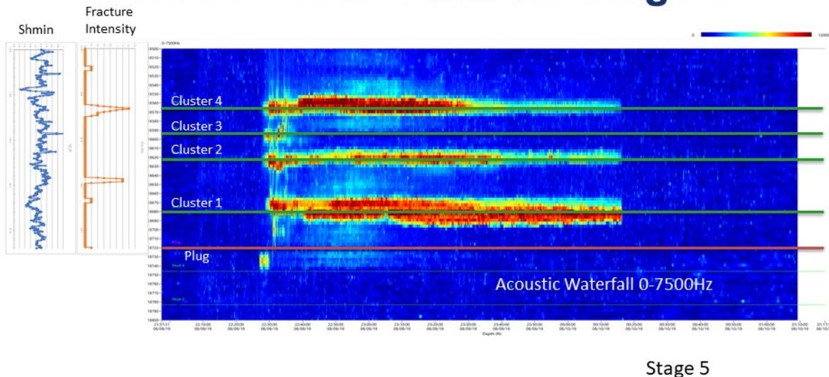
Figure 1.6: DAS data for Stage 5 showing four clusters and an uneven completion between clusters as indicated by acoustic amplitude recorded by the DAS. Cluster 3 received almost no stimulation and even cluster 2 is different than cluster 1 which received most of the sand and water.
