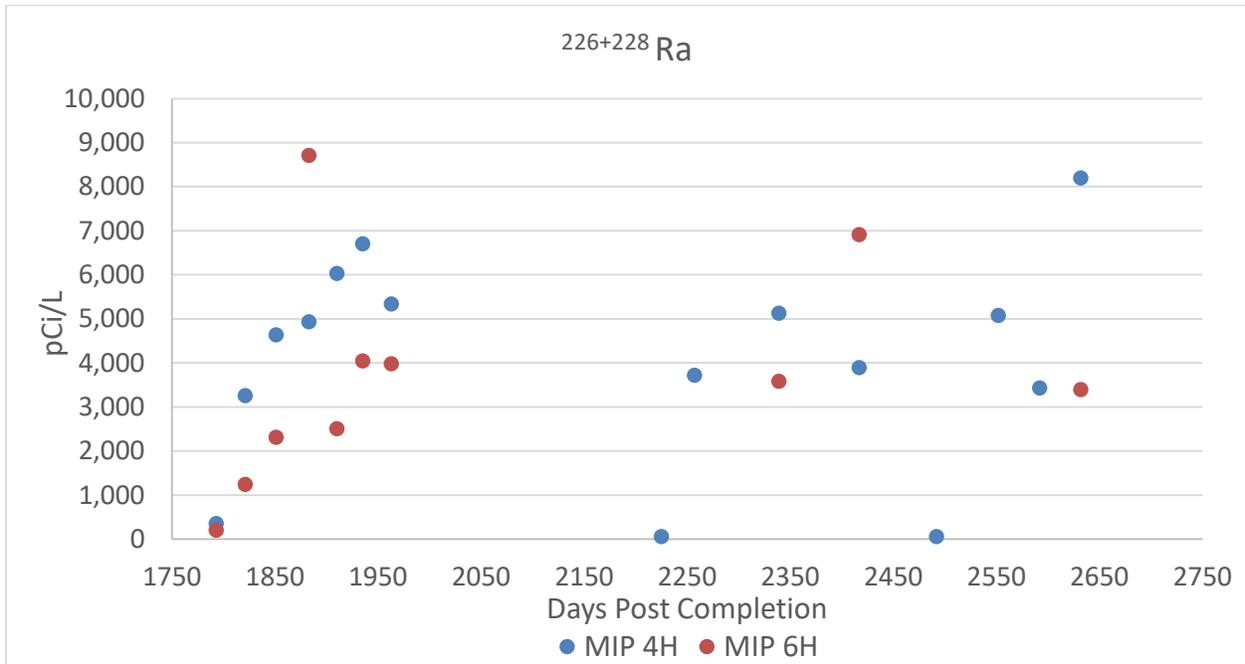
**Figure 4.6. The radium isotopes are plotted against days post well completion. Well 4H and 6H were choked at day 1963. At day 2225, 4H was reopened showing a value of 58 pCi/L and reopened again at day 2492 showing a value of 57 pCi/L.**
