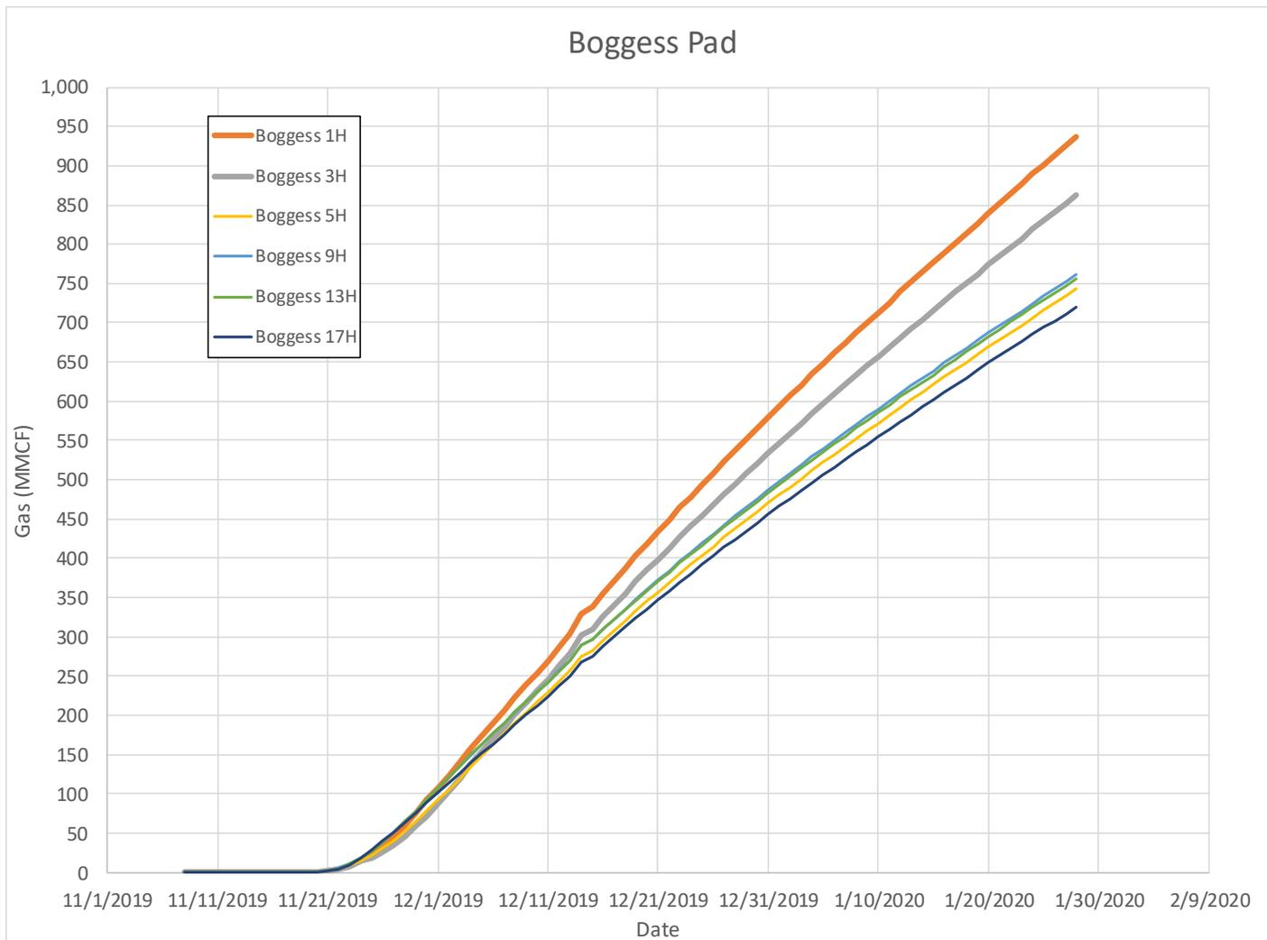
**Figure 1.2: Initial daily gross production from the Boguess Pad. The wells engineered using the MSEEL software are highlighted with thicker lines (1H and 3H). Wells have different lateral lengths that need to be evaluated to derive a better evaluation of production efficiency. Also outside wells typically perform better than interior wells due to reduced competition. The production is very early and the picture could very easily change.**
