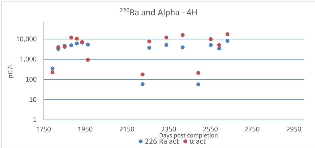
**Figure 4.9. The relationship between gross alpha and  $^{226}\text{Ra}$  as a function of time post completion at 4H.**
