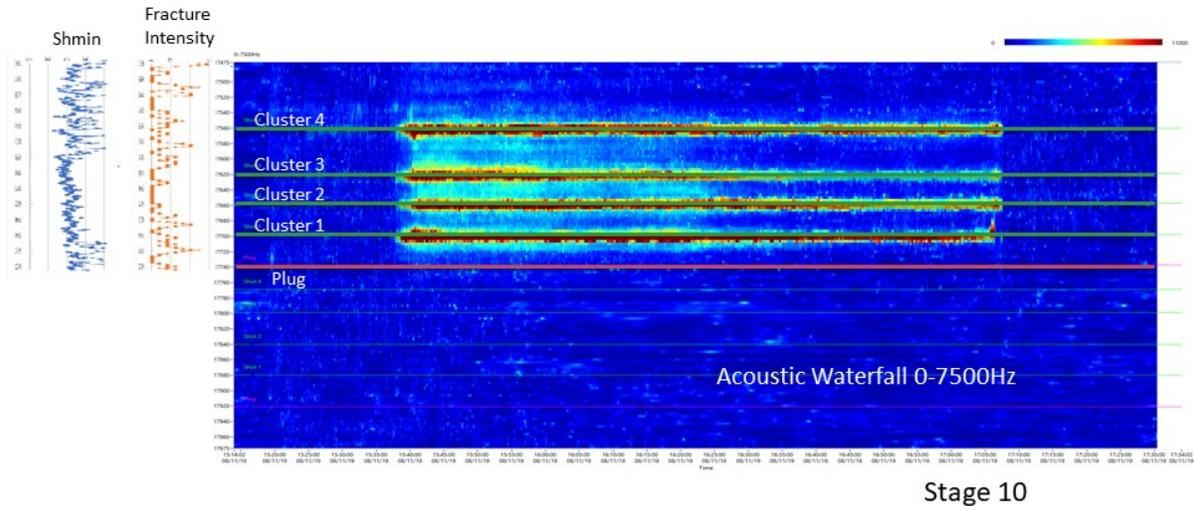
Figure 1.5: DAS data for Stage 10 showing four clusters and a consistent completion between clusters as indicated by acoustic amplitude recorded by the DAS.
