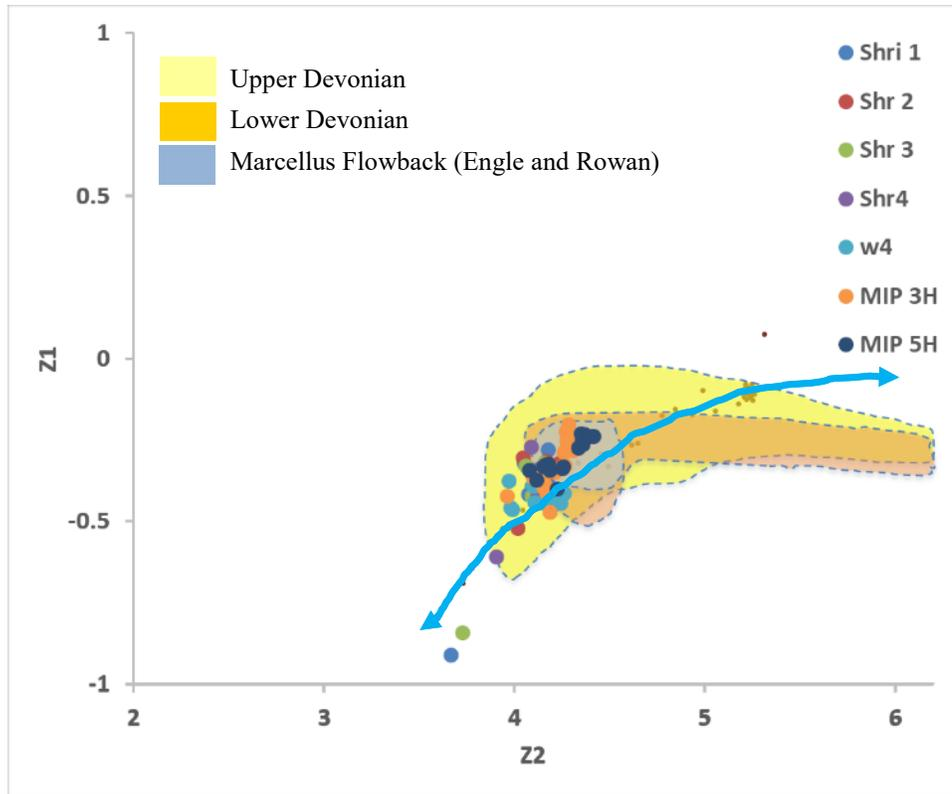
**Figure 3.1** ilr plot (Na-Cl-Br) redrafted after Engle and Rowan (2014) with flowback fluids from both the MSEEL site (MIP 3H and 5H) and the UPP wells (Shr 1-4 and W4). The blue line represents modern seawater evaporation pathway. The data plot along a trajectory that is consistent with evaporated paleo seawater.
