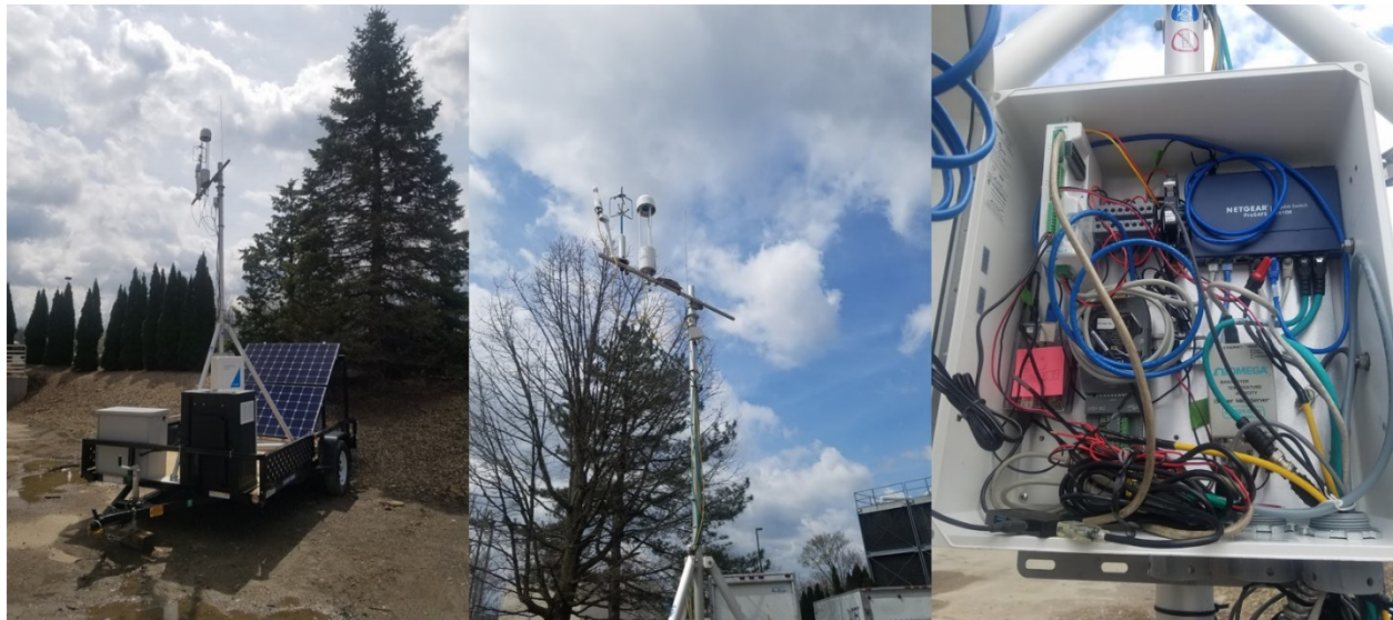
Figure 5.1: Completed eddy-covariance system for extended deployments.
