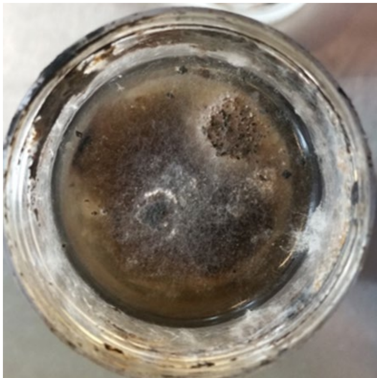
Figure 3-10 Microbial Activity on Pine Char Slurry after 205 Days
