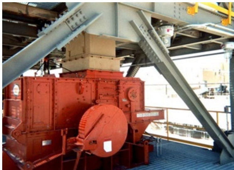
Figure 2-5 Typical Hammer Mill Installation
