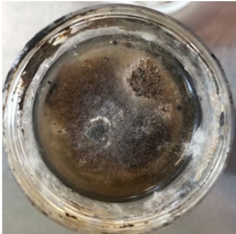
Figure 10 Microbial activity on pine char slurry after 205 days
