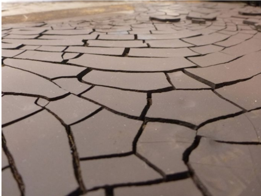
Figure 4-2 MRC Spill 24 Hours Later (From Hydrothermally Treated Lignite)
