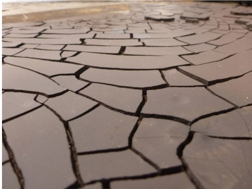
Figure 15 MRC spill 24 hours later (from hydrothermally treated lignite)
