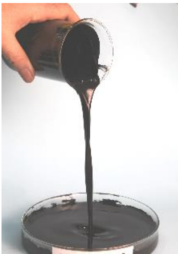
Figure 1-1 Typical MRC slurry
