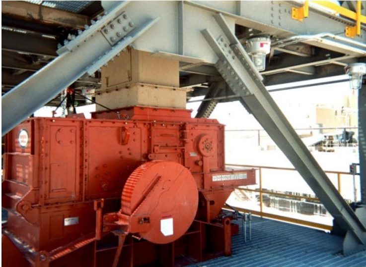
Figure 5-1 Typical hammer mill installation
