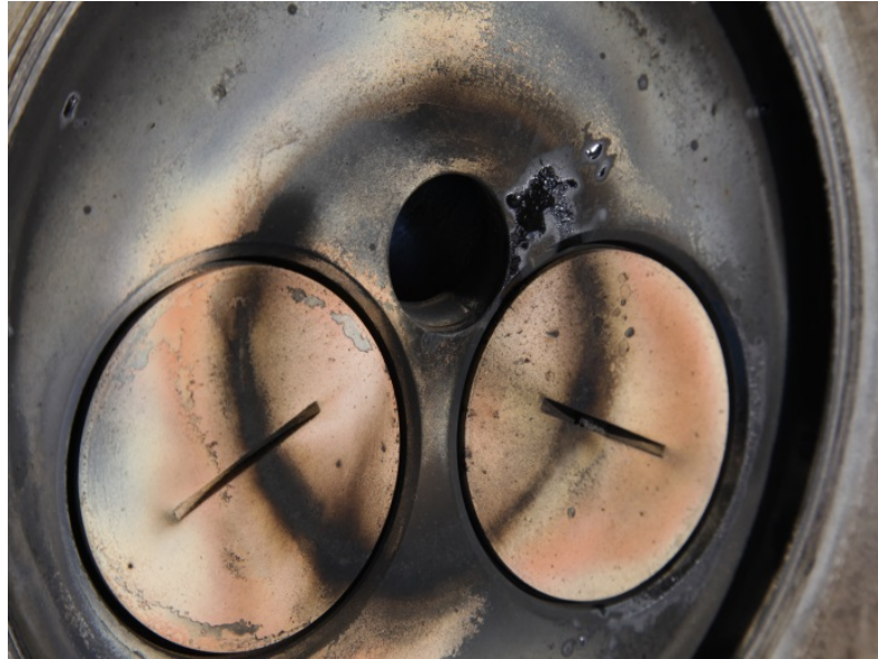
Figure 7 Head valves after 40 hours of full load operation using MRC produced from Yancoal UCC (courtesy Yancoal)
