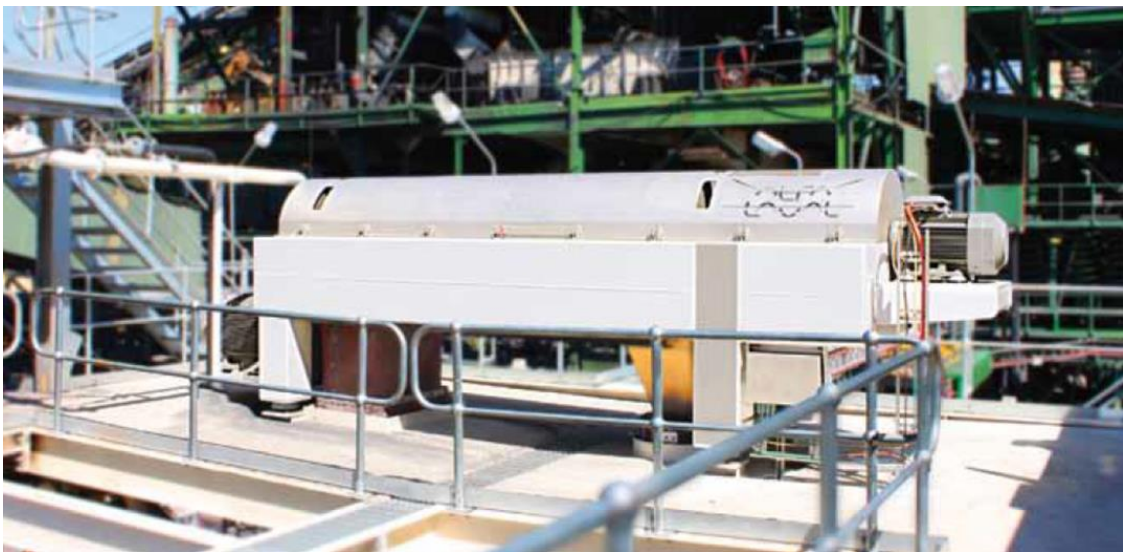
Figure 5-4 Typical Solidbowl Centrifuge Installation
