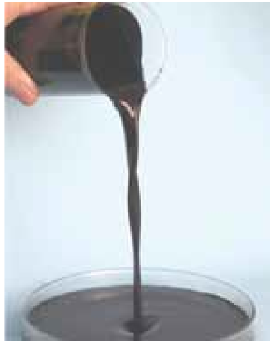
Figure 8 Fuel rheology. Left, coal water fuel for a boiler by JGC; right, MRC for DICE
