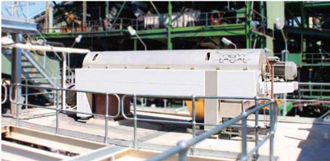
Figure 2-8 Typical Solid Bowl Centrifuge Installation
