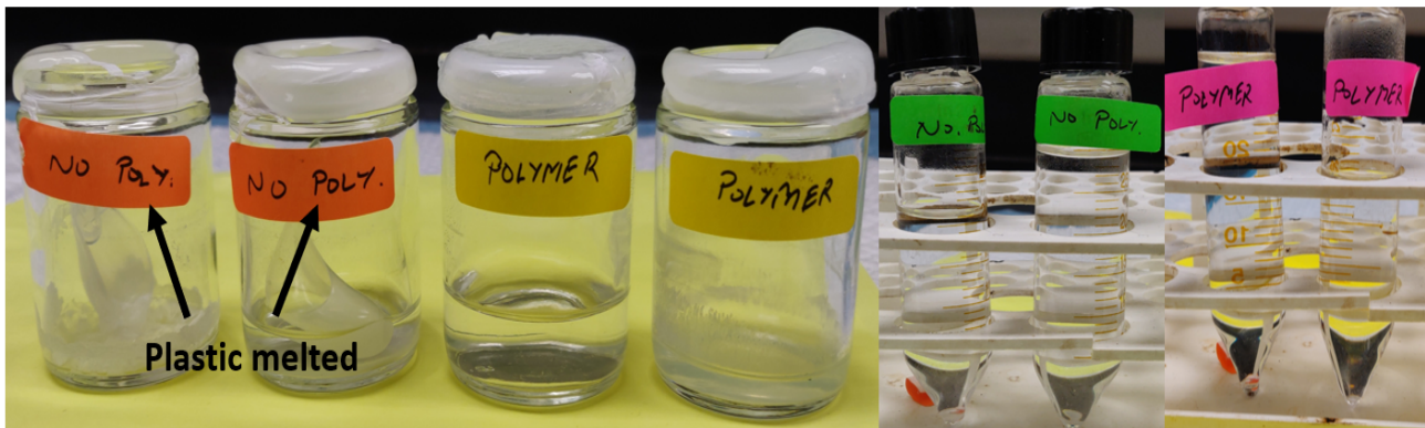
Figure 6.15: Cloud point test solutions after 4 hours at 240°F
