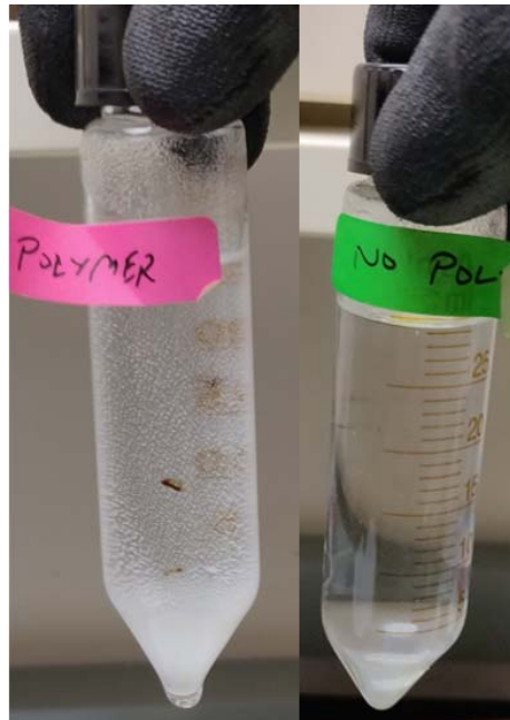
Figure 6.18: Cloud point test solutions after 12 hours at 250°F.
