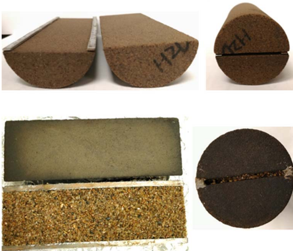
Figure 3.1: The sand-filled channeled core model
