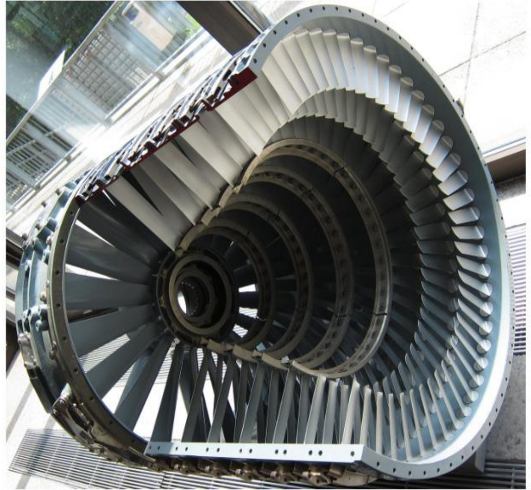
Left: Rotor of Siemens SGT5 series power gas turbine. (Courtesy of Siemens AG) Right: Stators of General Electric J79 aircraft engine (progenitor of LM1500 stationary gas turbines) on display at Deutsches Museum in Munich. (Credit: O. Cleynen).
