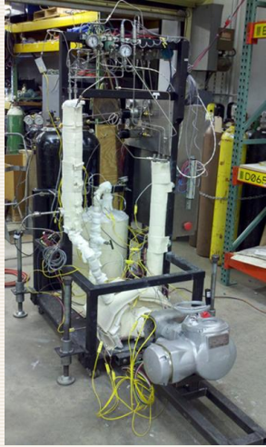
6 inch molten salt valve tests
