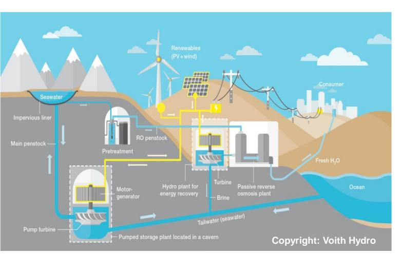
Seawater is pumped up into a lined upper reservoir using renewable energy sources
