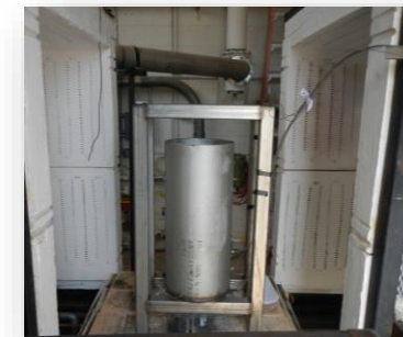
Small-scale hot-storage funnel-flow testing in a furnace
