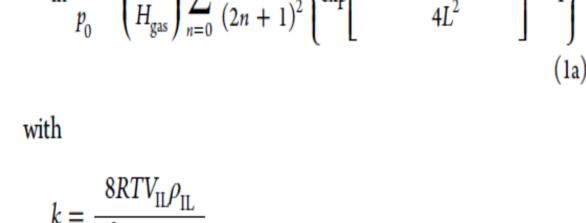
$E_a$  = activation energy (kJ/mol)  $D_{\rm gas}$  = diffusion coefficient of a gas in an ionic liquid (m<sup>2</sup> s<sup>-1</sup>)  $H_{gas}$  = Henry's Law constant of a gas in an ionic liquid (Pa)
