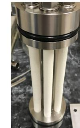
In-house developed zeolite membrane
