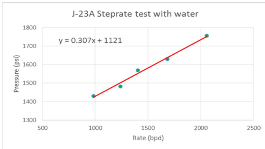
Figure 8. J-23A Pre-polymer step rate test results
