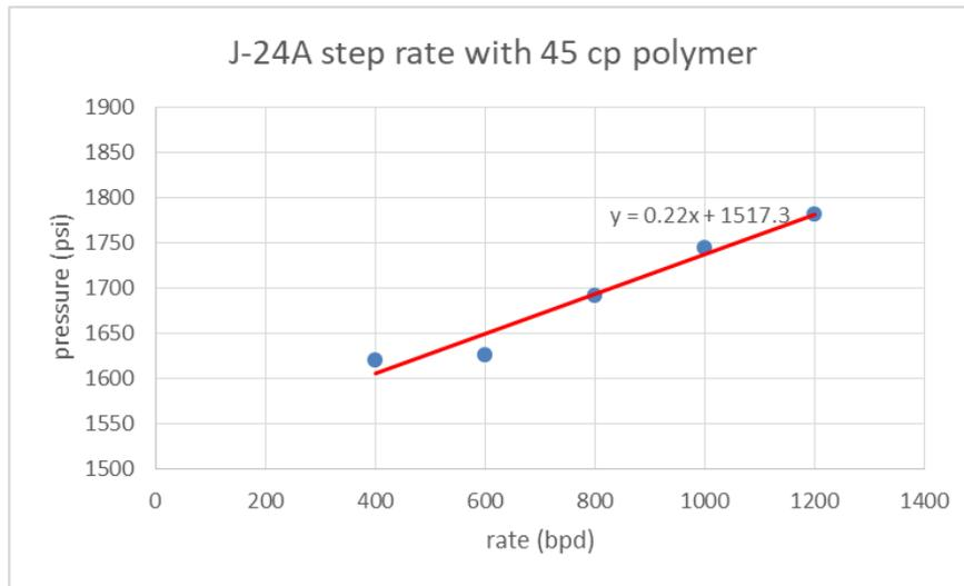
Figure 11. J-24A post-polymer step rate test results
