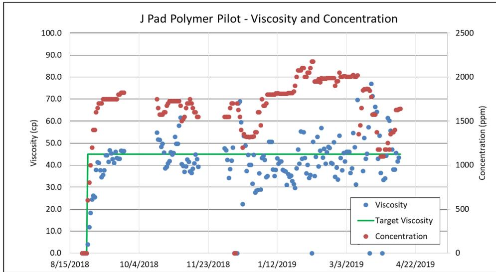
Figure 7. Polymer concentration and viscosity
