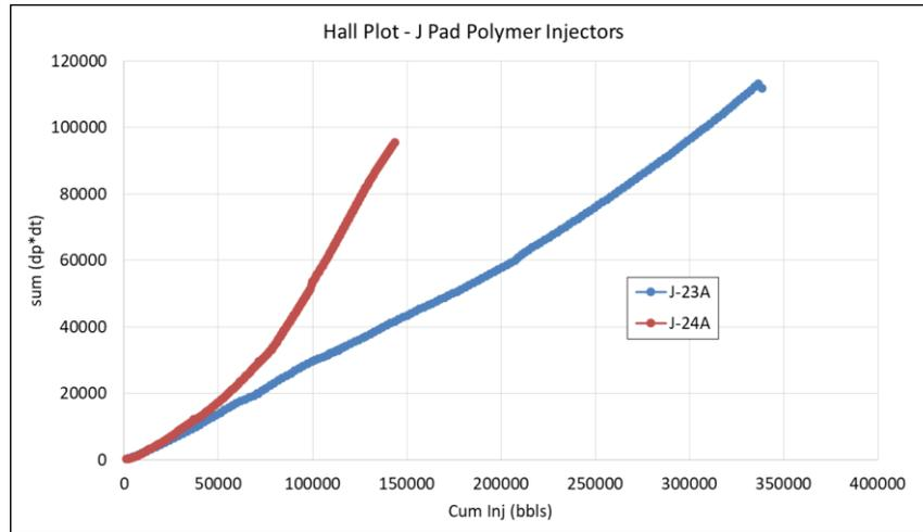
Figure 16. Hall plot during polymer injection
