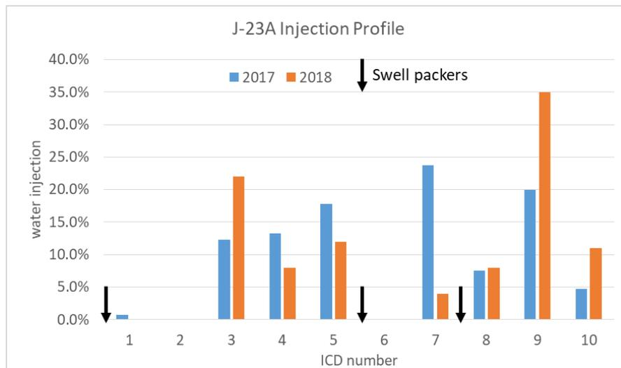
Figure 17. J-23A injection profile log
