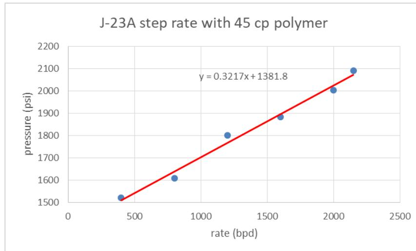
Figure 10. J-23A post-polymer step rate test results
