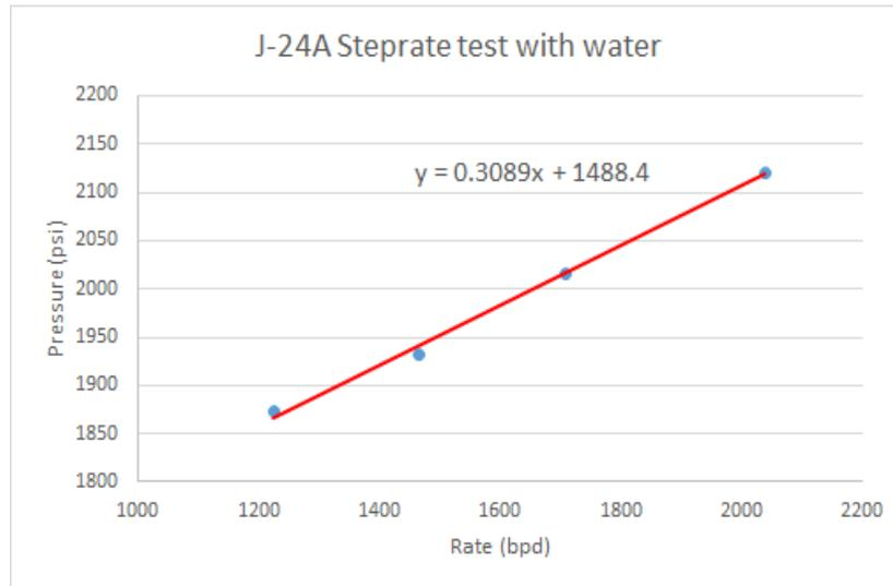
Figure 9. J-24A Pre-polymer step rate test results
