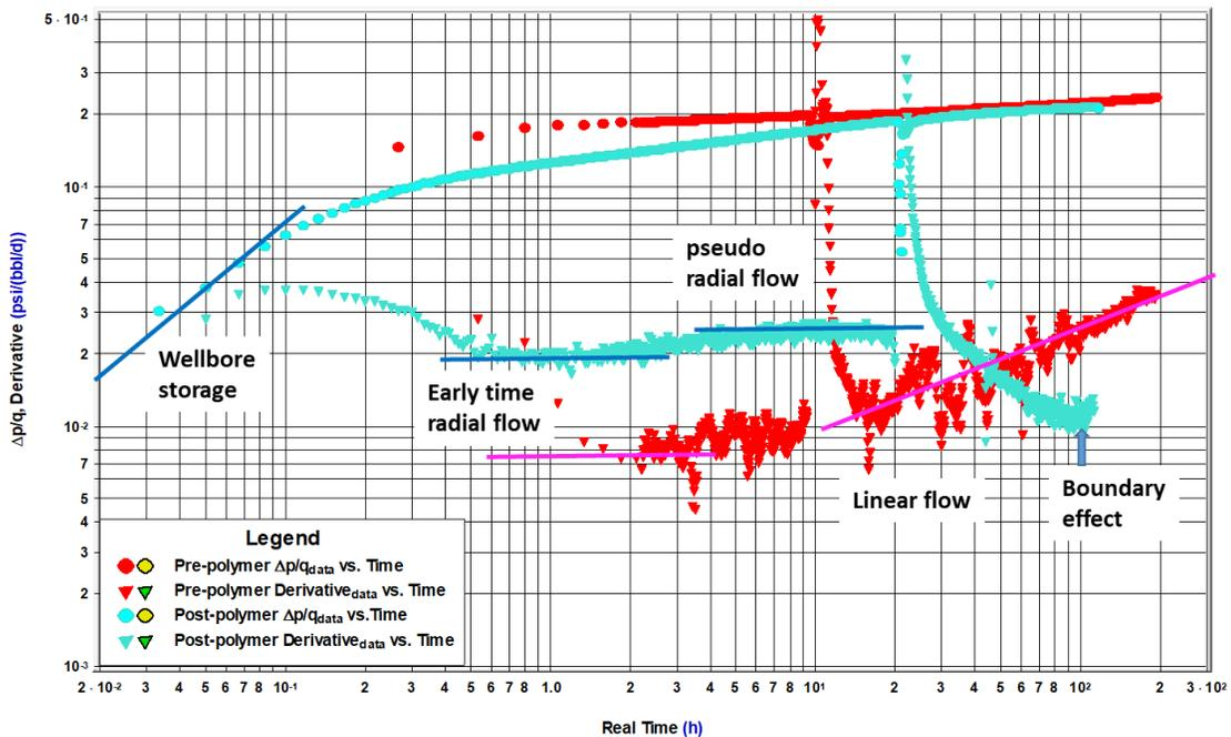
Figure 12. Comparison of J-23A pre and post-polymer PFO tests.
