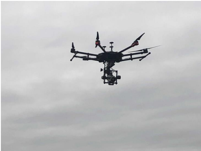
Figure 1. DJI Matrice 600 Pro carrying the OGI camera for data collection
