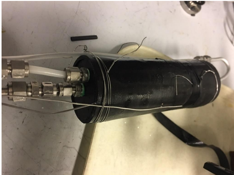
Fig 3.3.2. Packed elastomeric sleeve, showing inlet end cap with two inlets, a central one for fluid flow and temperature measurement, the other to accommodate the three capillary sensors.
