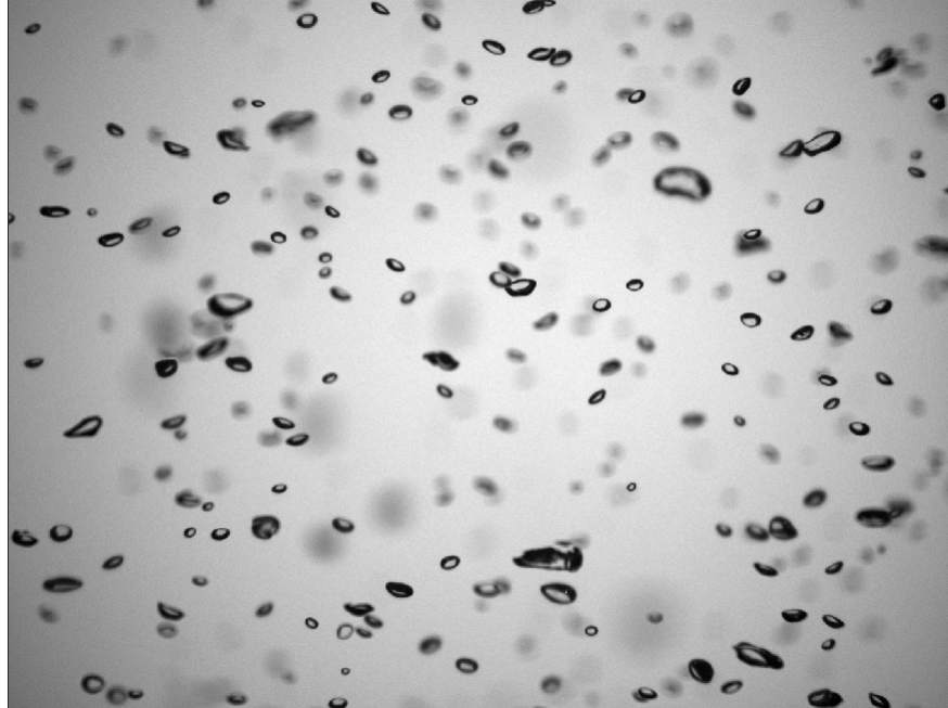
Figure 4: CCD video camera image of an airstone bubble plume at 3.0 NL/min gas flow rate at 11.45 m above the source.
