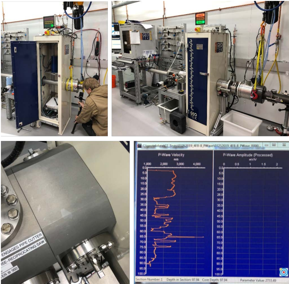
Figure 1-7. Top: Images of the new CT scanning attachment installed on the UT Mini-PCATS system, bottom: Images of the P-Wave attachment and initial data.
