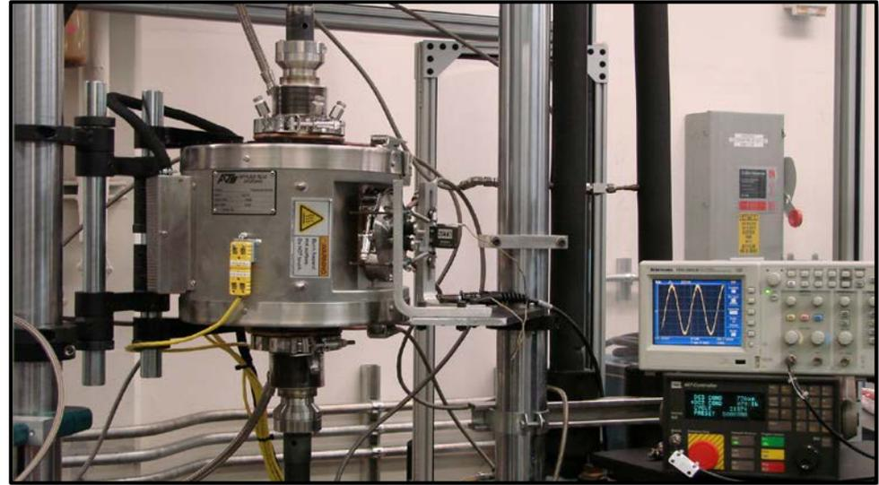
Sealed chamber inside furnace and extensometer to provide feedback signal for system operation under strain control
