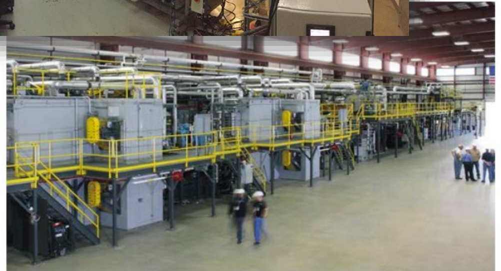
The carbon fiber pilot production line at Oak Ridge National Laboratories (ORNL, Oak Ridge, Tennessee) has provided fertile ground for the development of technologies that are helping make carbon fiber manufacture more efficient and less expensive. (Photo from Harper International – Pilot Line in operation at ORNL)
