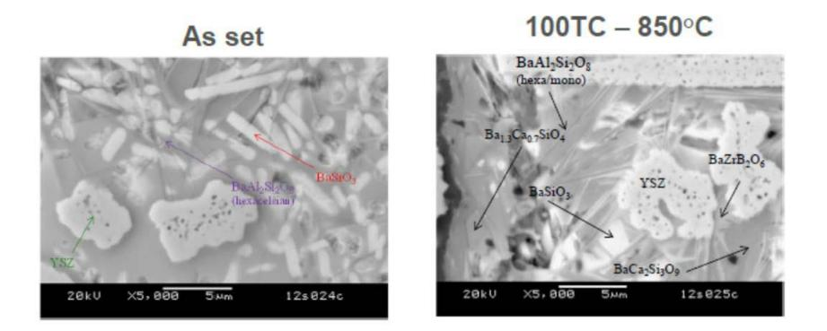
SEM with EDS used to identify phases formed in glass ceramic
