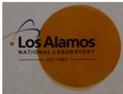
Cast 10 to 50 µm PBI in inert atmosphere
