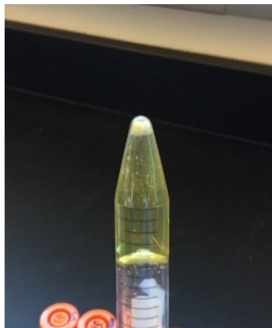
Gel formation in gluconic acid leachate of WY ash
