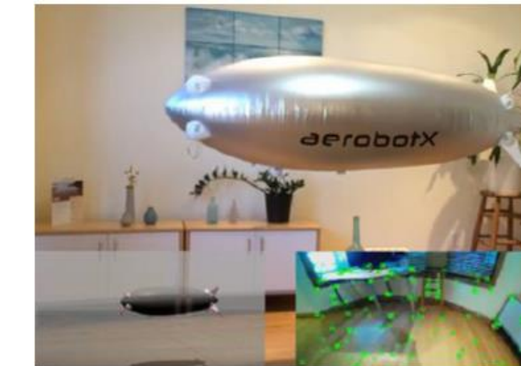
Fig. 1b. Lighter-than-air low thrust airship (courtesy: industrial partner, AerobotX)
