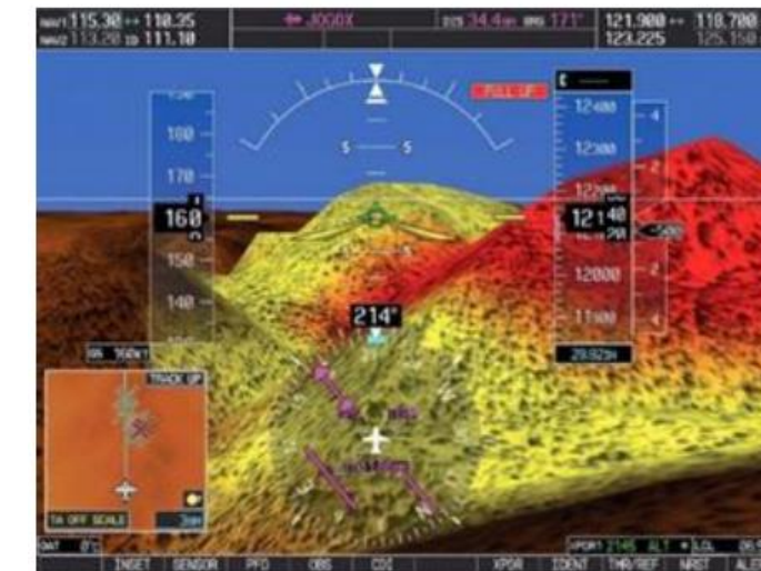
Fig. 1a. Synthetic vision (GARMIN Synthetic Vision Technology)
